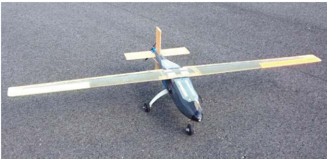
Figure 9. Split Wing 35% Scale Prototype in Forward Flight Configuration.
