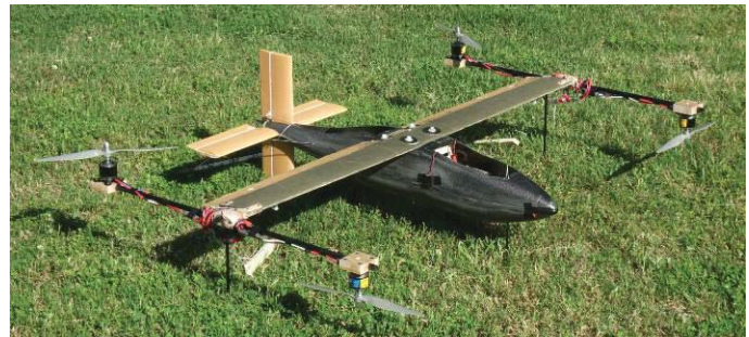
Figure 10. Split Wing 35% Scale Prototype in Hover Configuration.
