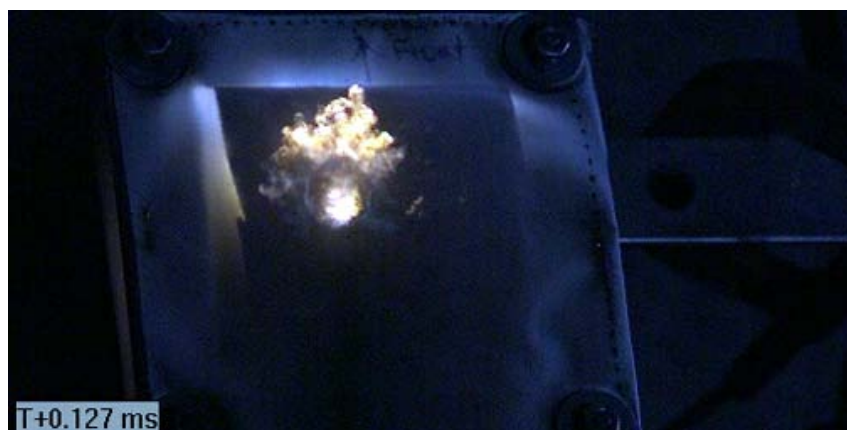
Figure C.8: Phantom v711 video image of projectile impacting Test #6B article
