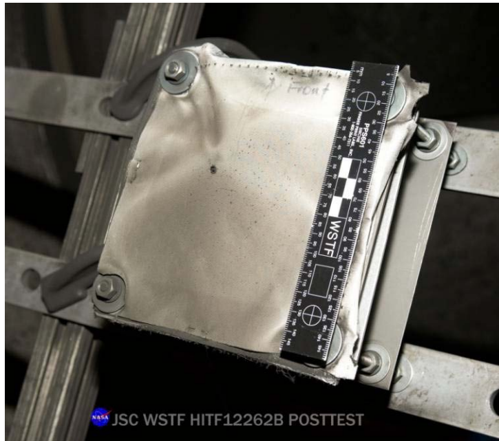
Figure 98: Post-test of ISS Soyuz Orbital Module Test #6B (HITF12262) article mounted in 0.50-caliber target tank.
