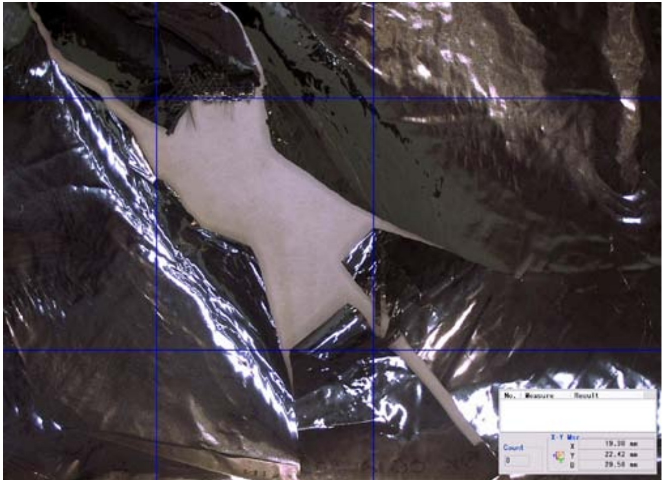
Figure 135: Mylar Film Layer 2 of ISS Soyuz OM Test #8 (Keyence 3D Microscope Image)
