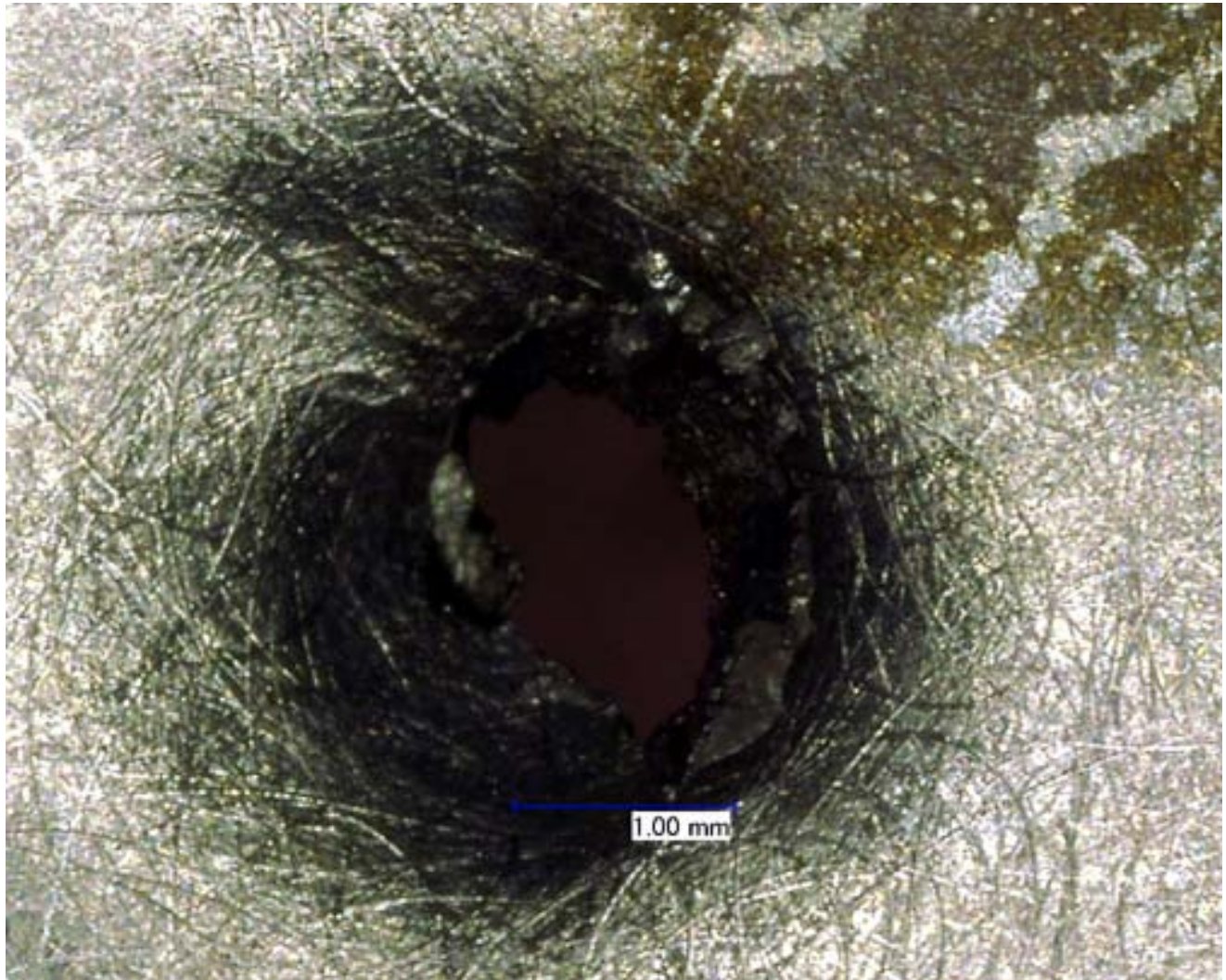
Figure 126: AI 5456-0 Rear Wall Layer 8 Back of ISS Soyuz OM Test #7 (Keyence 3D Microscope Image)
