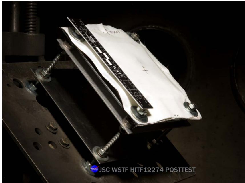
Figure 232: Post-test of ISS Soyuz Orbital Module Test #14 (HITF12274) article mounted in 0.17-caliber target tank.
