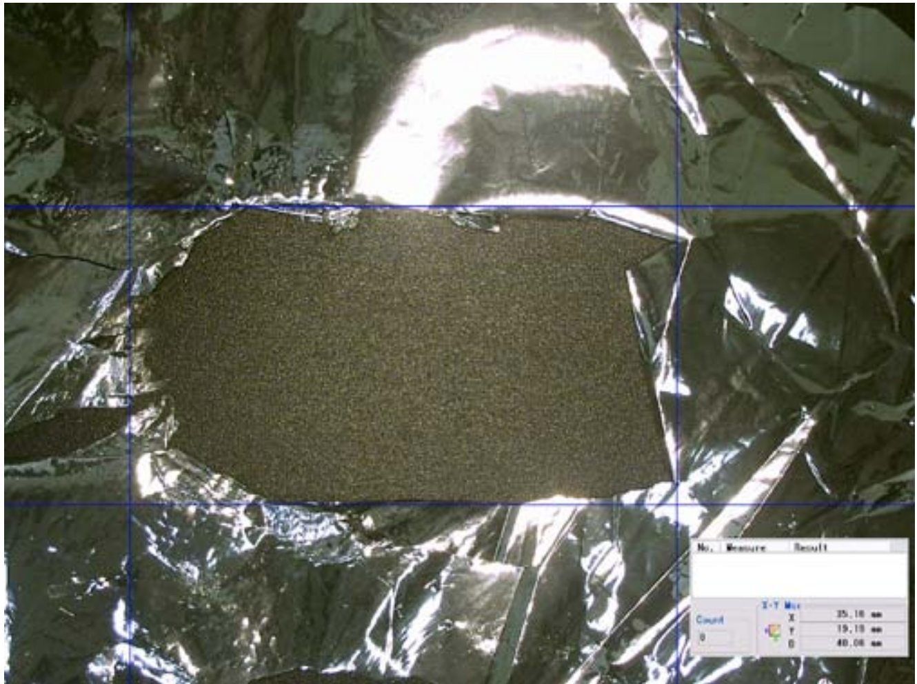
Figure 151: Mylar Film Layer 2 of ISS Soyuz OM Test #9 (Keyence 3D Microscope Image)
