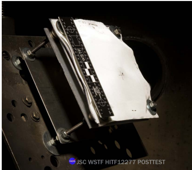
Figure 280: Post-test of ISS Soyuz Orbital Module Test #17 (HITF12277) article mounted in 0.17-caliber target tank.
