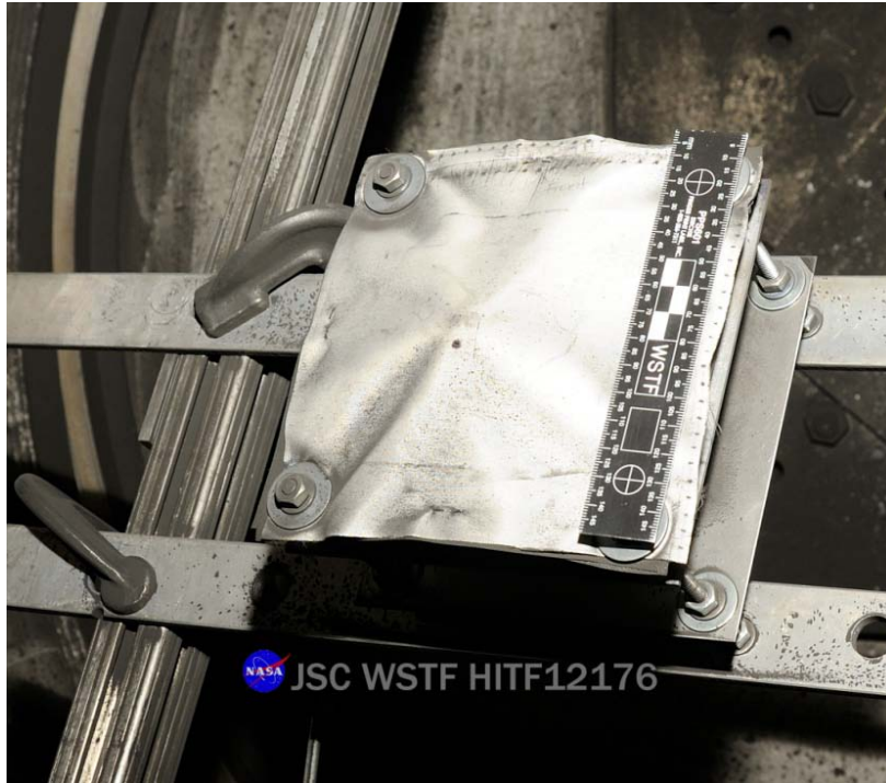
Figure 264: Post-test of ISS Soyuz Orbital Module Test #16 (HITF12276) article mounted in 0.50-caliber target tank.
