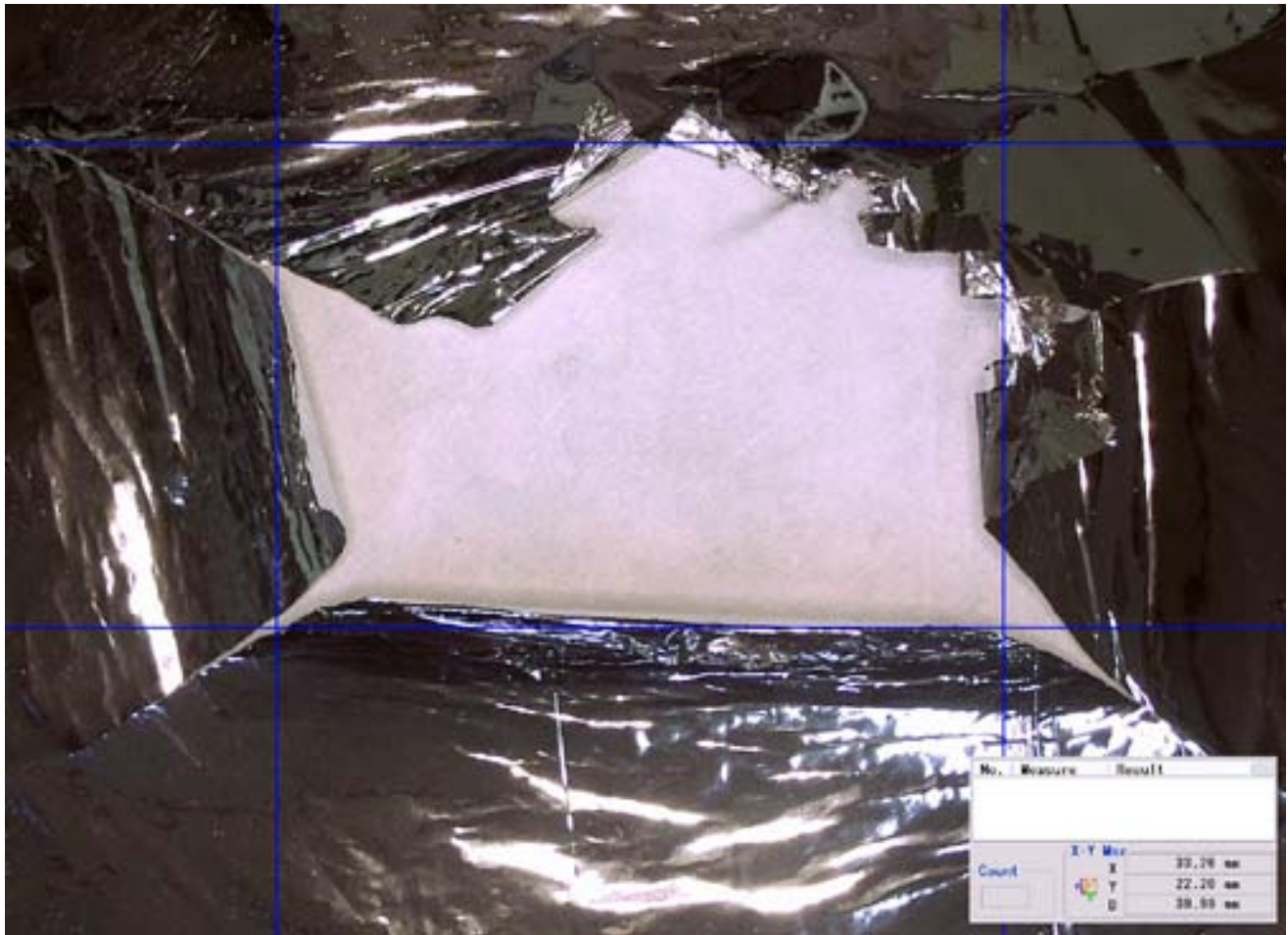
Figure 236: Mylar Film Layer 2 of ISS Soyuz OM Test #14 (Keyence 3D Microscope Image)
