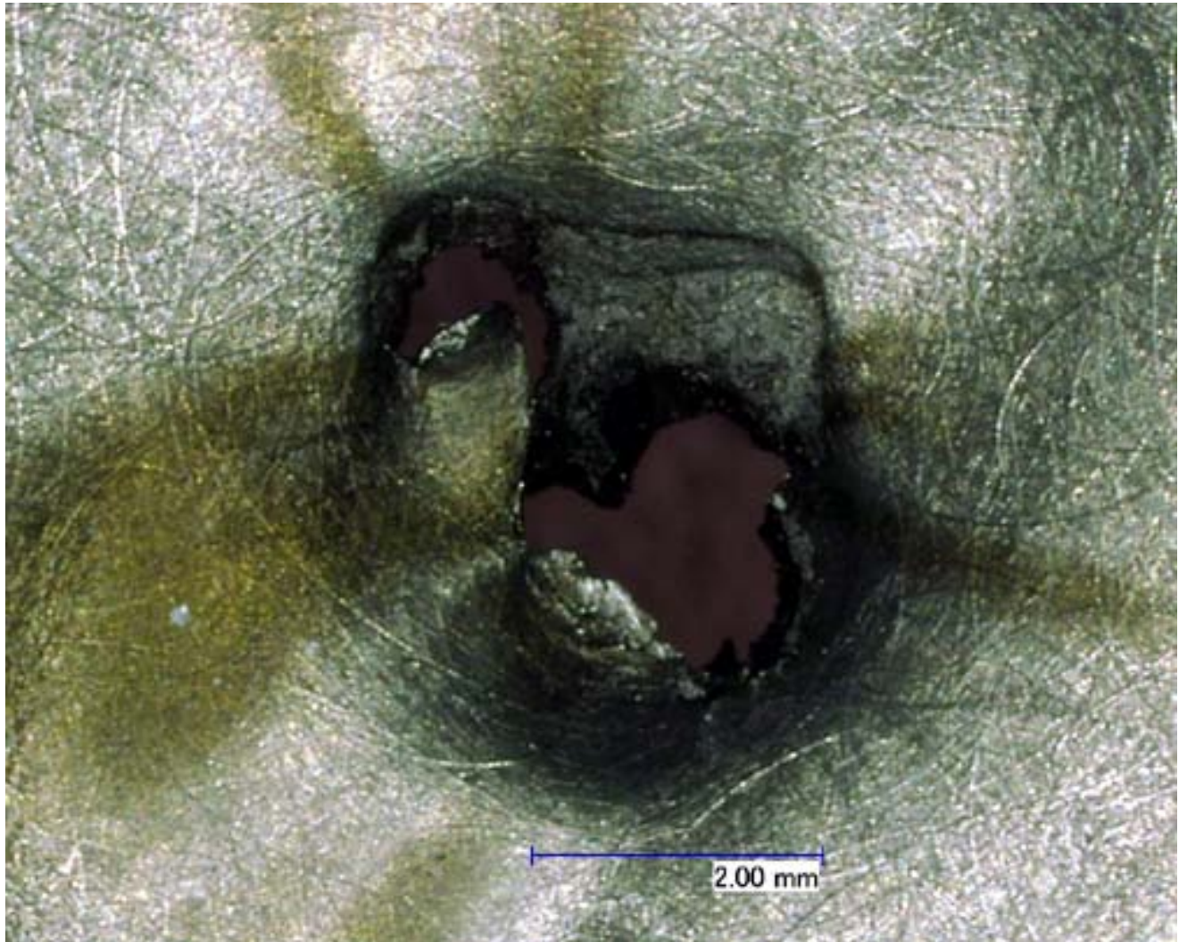
Figure 62: Al 5456-0 Rear Wall Layer 8 Back of ISS Soyuz OM Test #3 (Keyence 3D Microscope Image)
