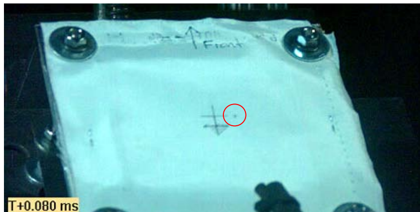
Figure C.23: Test #12 Phantom v711 high speed video image of projectile prior to impact
