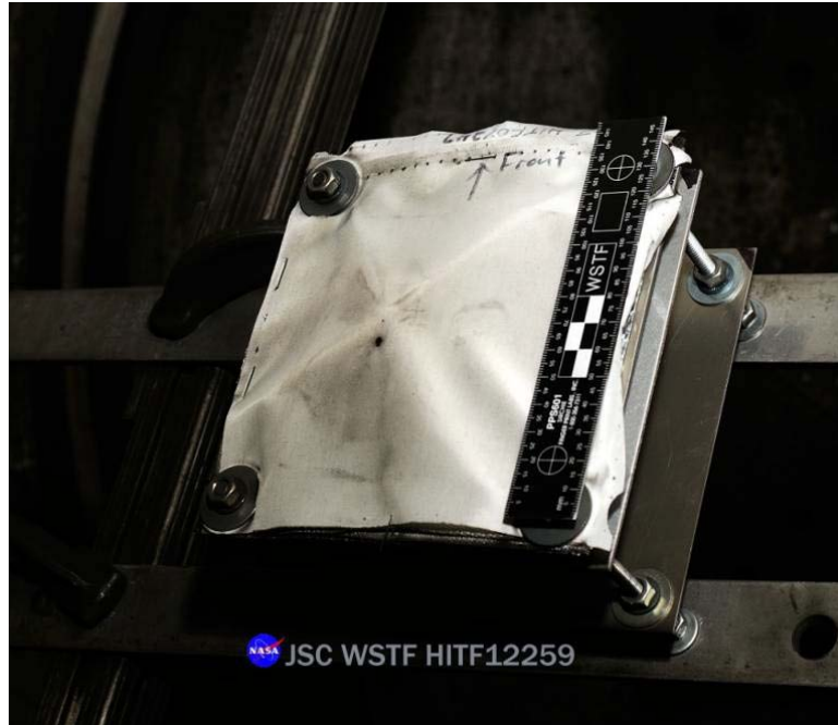
Figure 50: Post-test of ISS Soyuz Orbital Module Test #3 (HITF12259) article mounted in 0.50-caliber target tank.
