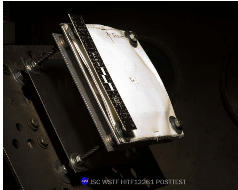
Figure 83: Post-test of ISS Soyuz Orbital Module Test #5 (HITF12261) article mounted in 0.17-caliber target tank.
