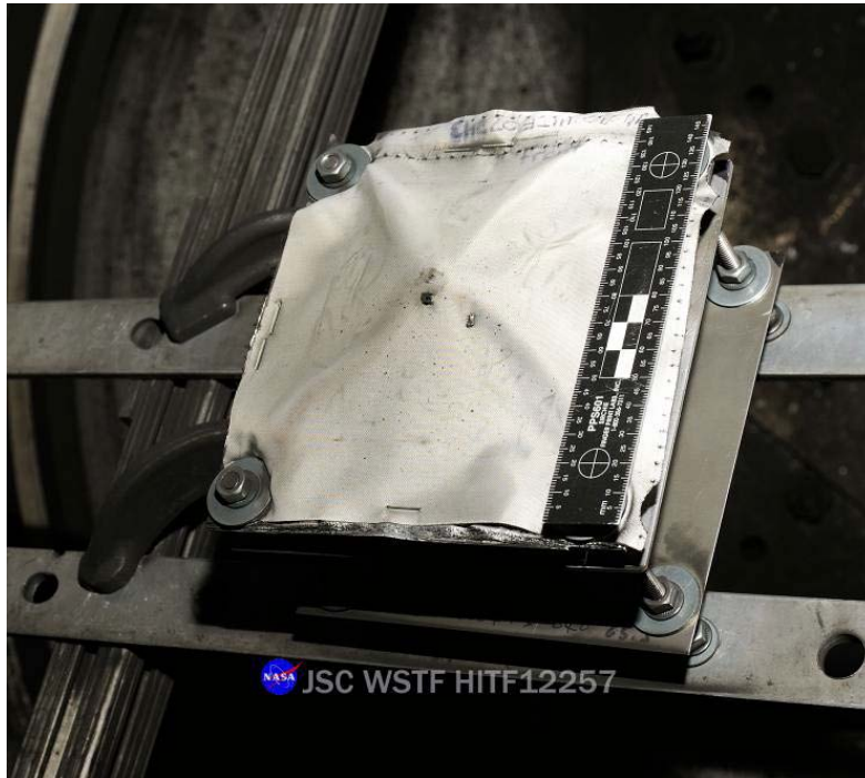
Figure 16: Post-test of ISS Soyuz Orbital Module Test #1 (HITF12257) article mounted in 0.50-caliber target tank.
