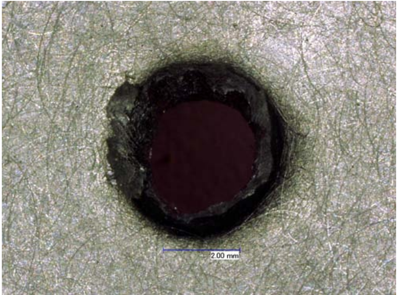
Figure 174: Al 5456-0 Rear Wall Layer 8 Back of ISS Soyuz OM Test #10 (Keyence 3D Microscope Image)
