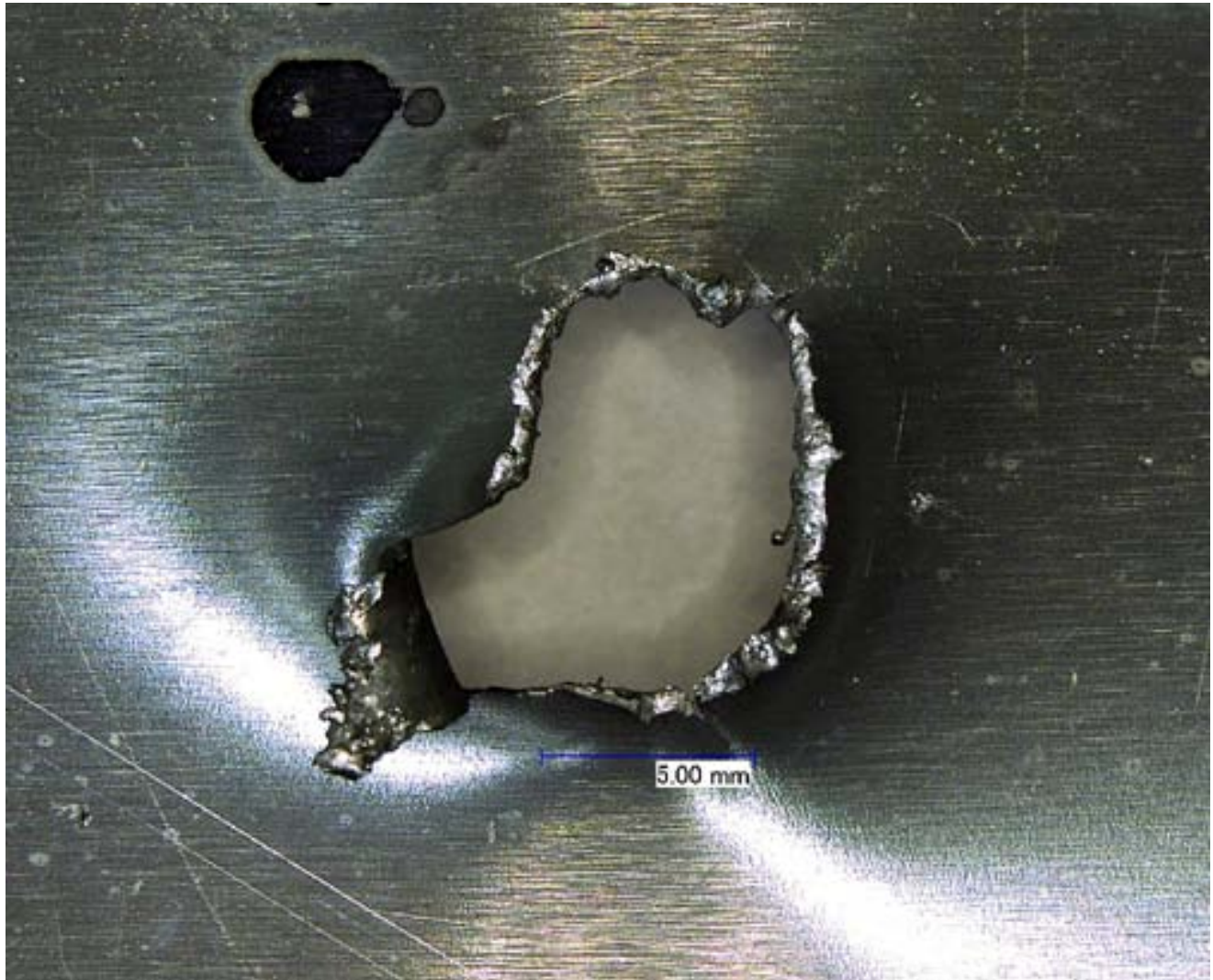
Figure 157: Al 6061-T6 Layer 7 Back of ISS Soyuz OM Test #9 (Keyence 3D Microscope Image)
