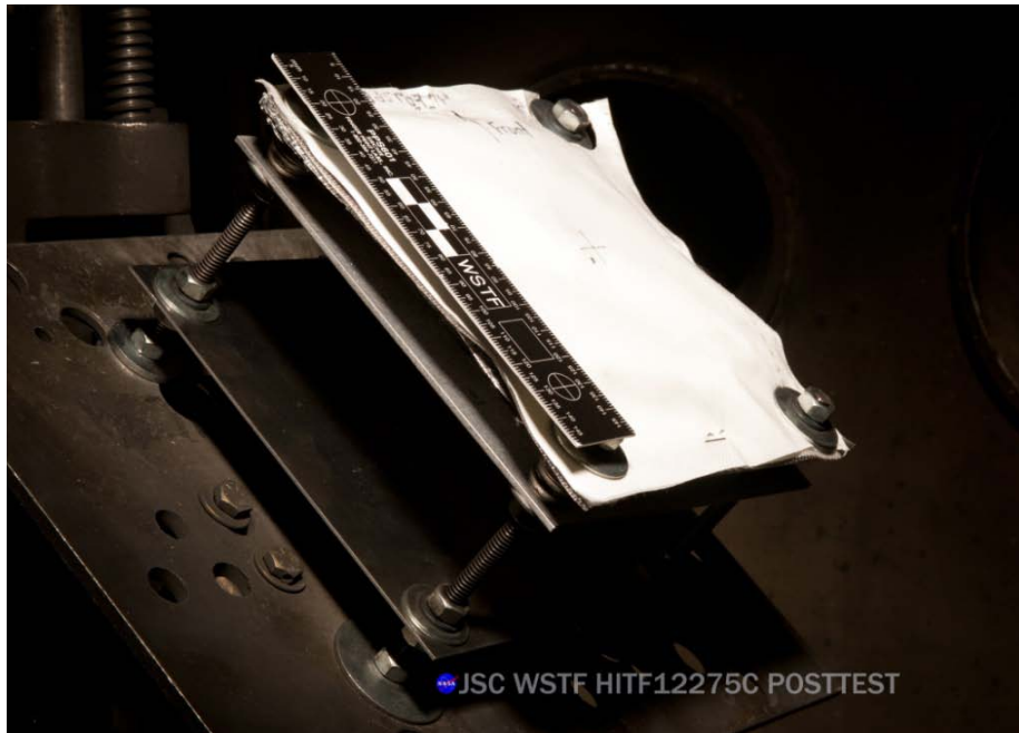
Figure 250: Post-test of ISS Soyuz Orbital Module Test #15C (HITF12275) article mounted in 0.17-caliber target tank.
