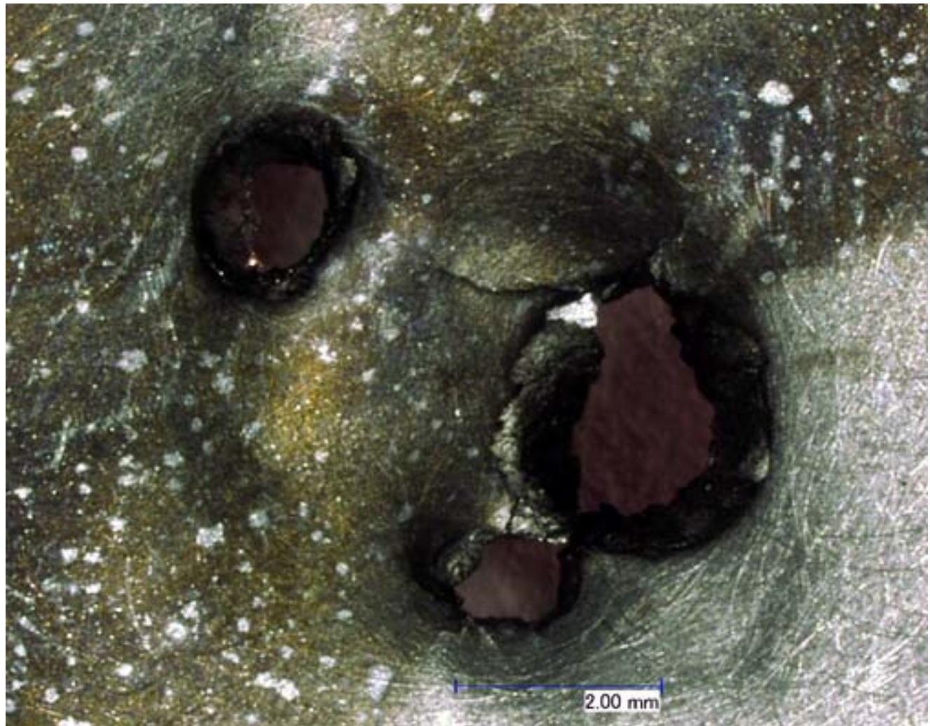
Figure 28: Al 5456-0 Rear Wall Layer 8 Back of ISS Soyuz OM Test #1 (Keyence 3D Microscope Image)
