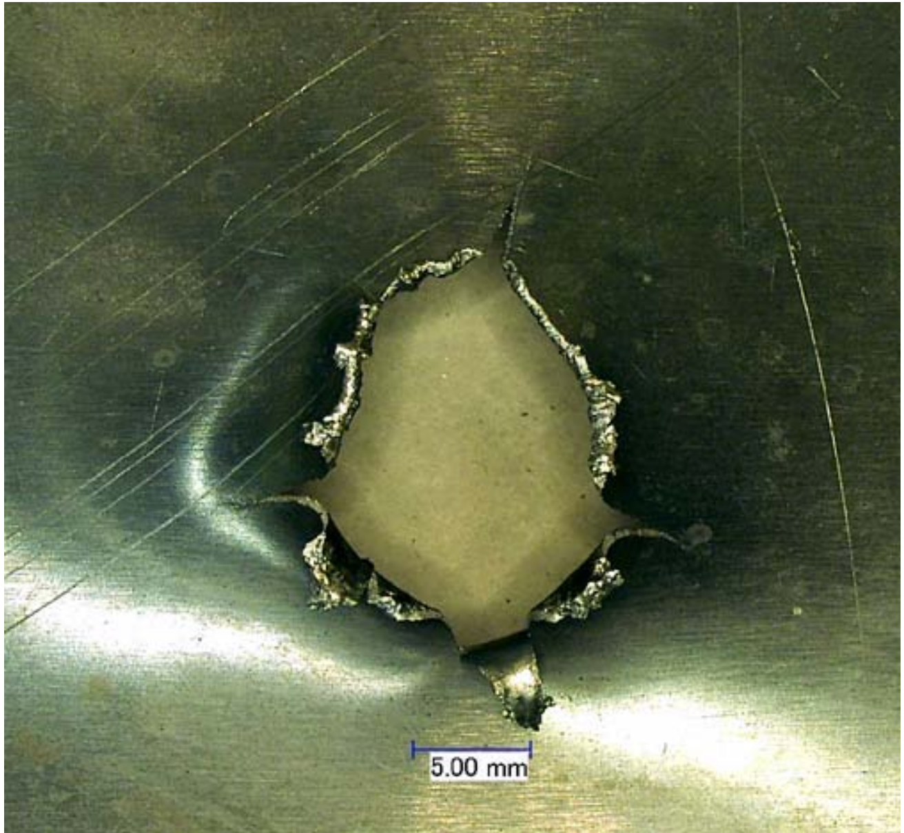
Figure 76: Al 6061-T6 Layer 7 Back of ISS Soyuz OM Test #4 (Keyence 3D Microscope Image)
