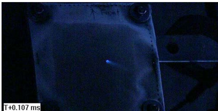
Figure C.7: Test #6B Phantom v711 high speed video image of projectile prior to impact
