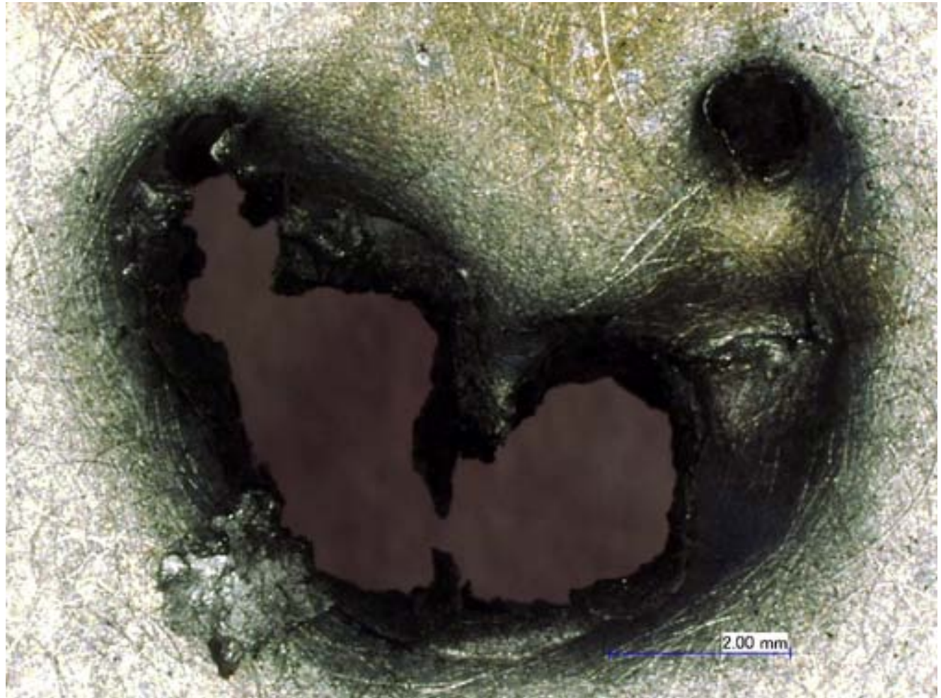
Figure 45: Al 5456-0 Rear Wall Layer 8 Back of ISS Soyuz OM Test #2 (Keyence 3D Microscope Image)
