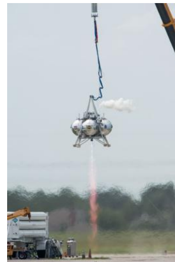
Figure 7 – Morpheus 1.5 ‘Bravo’ executing a Tether Test in July 2013
