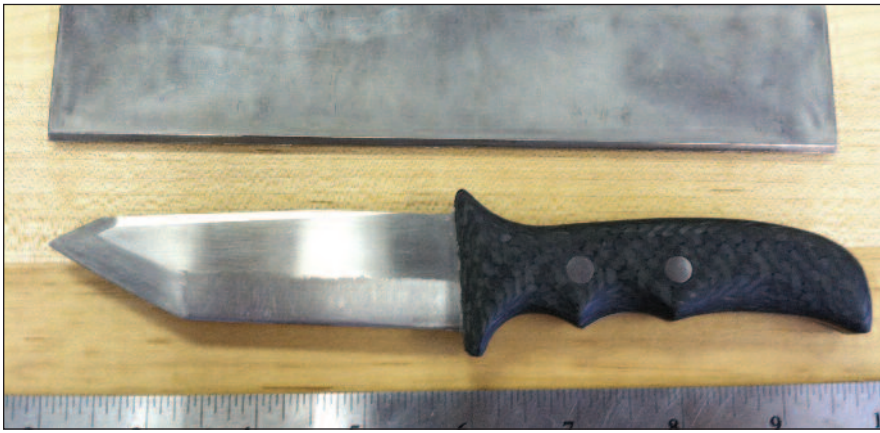
A full tang Bulk Metallic Glass Tactical Knife with multi-faceted blade surface and carbon fiber grip with titanium pins, fabricated by Benjamin Potter of Altadena, CA. The knife was fabricated by water-grinding from a larger plate as an illustration. In a commercial setup, the knife would be cast to a net-shape using an auto-feed and eject system, similar to what is done in plastics.
