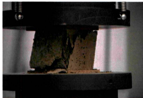
Figure 5. Crushed test specimen after failure
