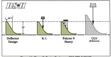
Figure 11: Flame Deflector Design per KSC-STD-Z-0012B
