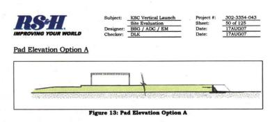
In Option A, shown above, the flame deflector is completely above grade and the integration building is elevated to provide a flat horizontal transportation route. Having the flame deflector completely above grade prevents water accumulation in the flame trench. This option requires the largest amount of fill due to the elevated integration building and the fill required to maintain that elevation all the way to the pad.
