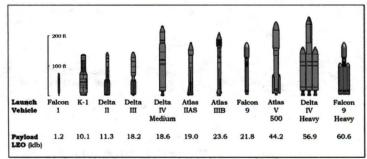
Figure 2: Relative US Launch Vehicle Sizes and Performance
