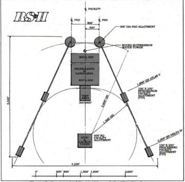
**Figure 7: Symmetrical Vertical Launch Facility Site Layout**
