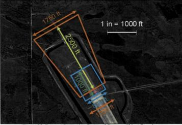
Figure 28: Runway Protection Zone and Runway Object Free Area
