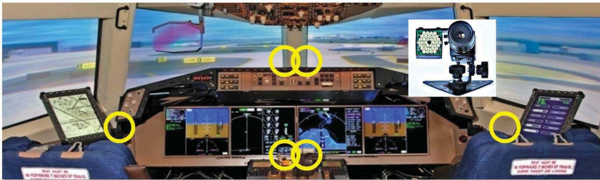
Figure 2. Head- and Eye-Tracking System Infrared Camera (inset) and Locations
