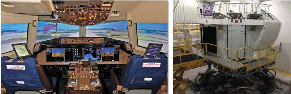
Figure 1. CMF/RFD Simulator (Note: For this study, the EFBs were re-positioned inboard and lower than shown; the right-side HUD is not shown.)
