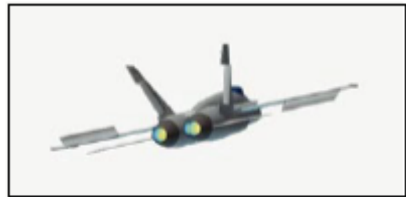
(d) Ailerons are deflected to bank the aircraft to the left to stabilize at a constant heading.
