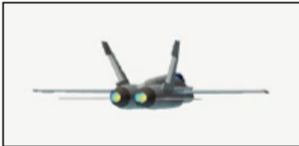
(c) Aircraft will yaw to the right in response to the rudder input.
