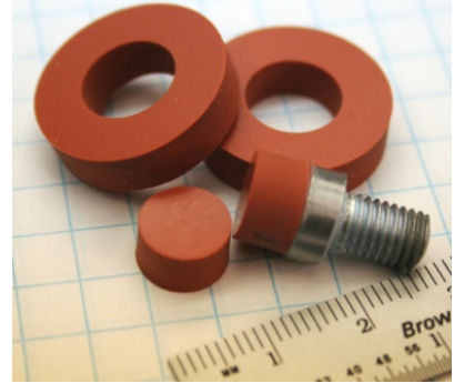
Figure 1.—Seals and buttons made from S0383-70 elastomer.
