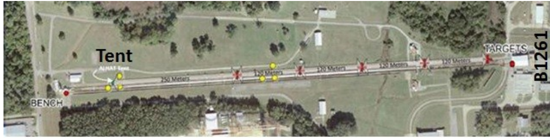
Figure 14. Flash Lidar accuracy calibration target layout on the LDTR with five targets from 250m to 730m spaced 120 meters apart.
