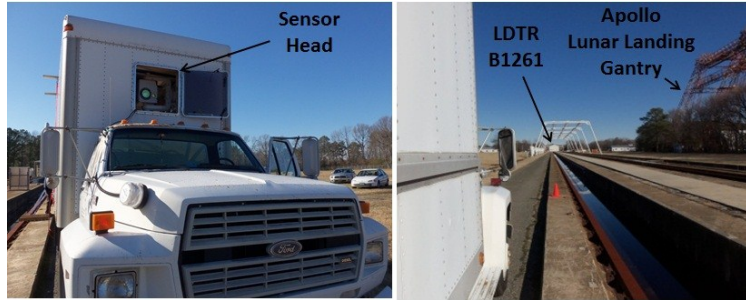
Figure 16. Flash Lidar during integrated ALHAT-Morpheus truck testing on the LaRC LDTR.
