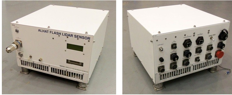
Figure 6. Gen 2.2 Flash Lidar Electronics Box (LEB) front and back.
