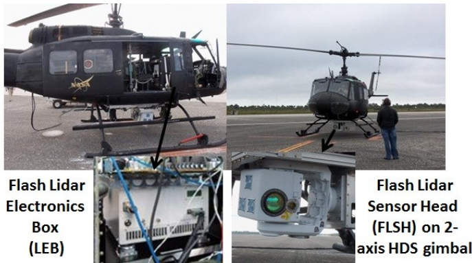
Figure 17. Flash Lidar integrated to LaRC UH-1H helicopter at rest on KSC Shuttle Landing Facility (SLF) runway.
