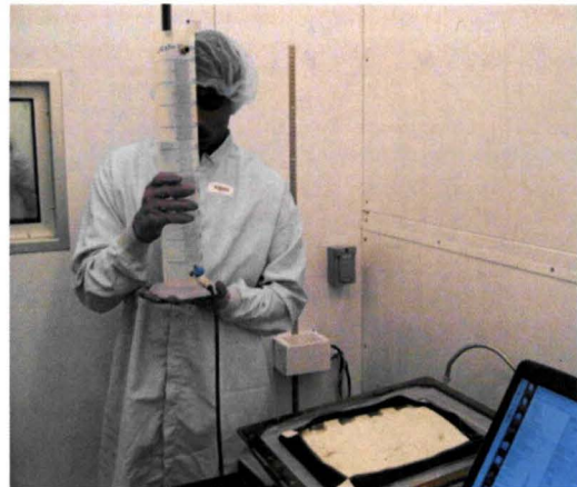
Figure 7: Graduated cylinder method
