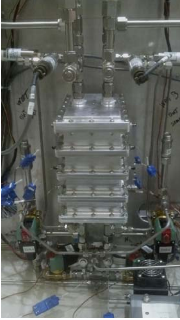
Figure 1. Sub-scale IBD test setup, with two beds, each with 4 cells.
