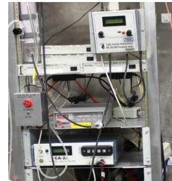
Figure 5. Major constituent analysis instrument array.
