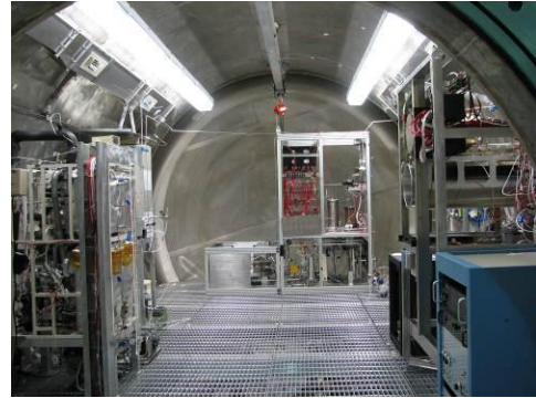
Figure 4. An EChamber interior view. Carbon dioxide removal (left), trace contaminant control (right), and oxygen generation equipment (rear) are visible.
