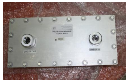
Figure 2. Proteus CO 2 removal membrane.
