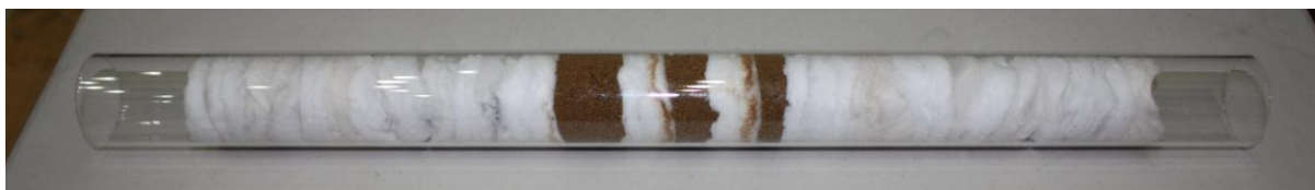
Figure 4. Unreacted Martian regolith simulant-packed reactor tube.
