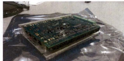
Figure 7. Elmo Motion Controller. The Elmo Duo motion controller was recommended by the HoneyBee Robotics lab.
