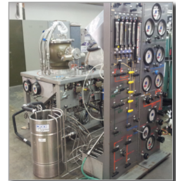
Prevalve Bench Testing on Common Cryo Test Stand
