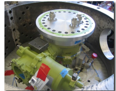
Fill & Drain Valve Test Setup
