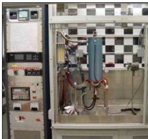
CVD particle Coating furnace
