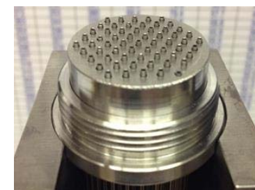
Above: 61 channel head with modified tooling to prevent bending in the tubes. Will use braze foil instead of braze paste.
