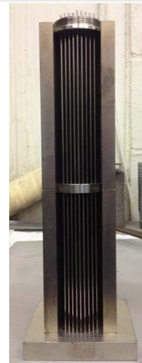
Complete front view of a 61-channel etch component just prior to the brazing process. This component will be used to chemically etch the coolant channels in a uranium dioxide-tungsten fuel element.
