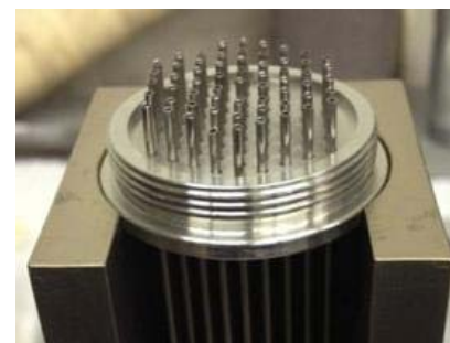
Top view of a 61-channel etch component just prior to the brazing process, showing the channel head and etch tubes positioned in the brazing assembly.
