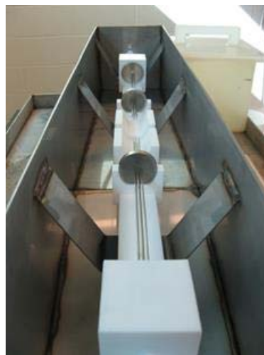
Top view of the chemical etching system configured to etch a 7-channel fuel element. The 7-channel fuel elements will be tested in CFEET.
