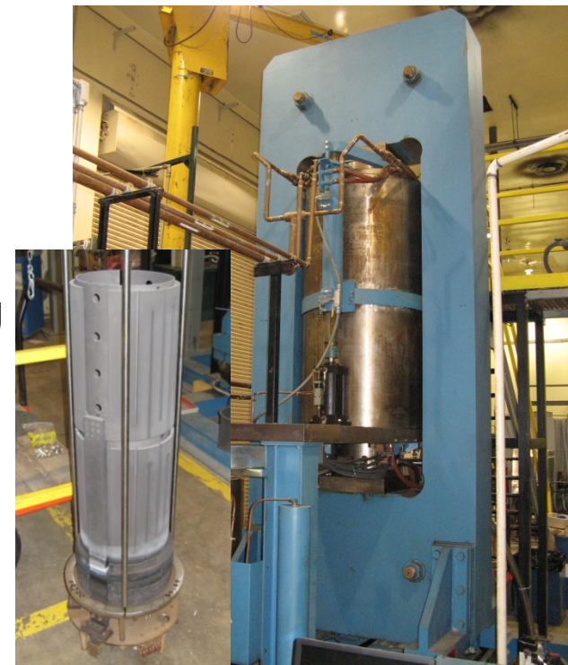
MSFC HIP pressure vessel (right). Graphite furnace removed (left).
