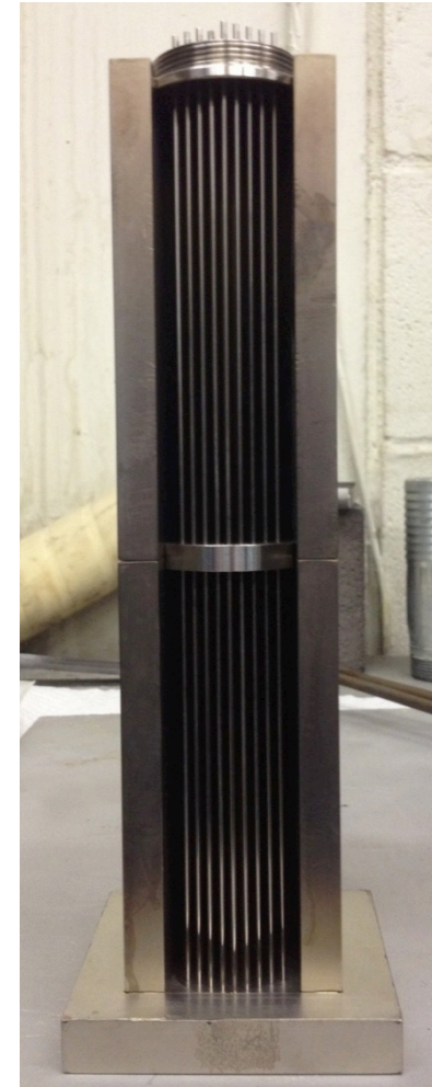
Complete front view of a 61-channel etch component just prior to the brazing process. This component will be used to chemically etch the coolant channels in a uranium dioxide-tungsten fuel element.
