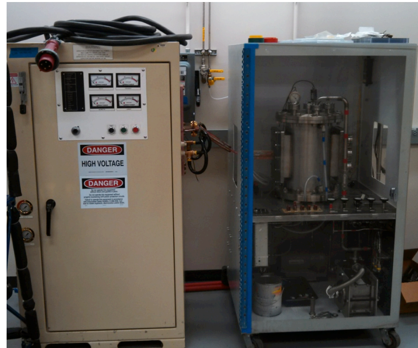
50kW power supply and containment
