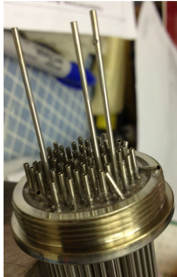
Front view of the chemical etching system. The system is designed to etch 7-channel and 61-channel fuel elements which will be tested in the Compact Fuel Element Environmental Tester (CFEET), and in the Nuclear Thermal Rocket Environmental Element Simulator (NTREES).
