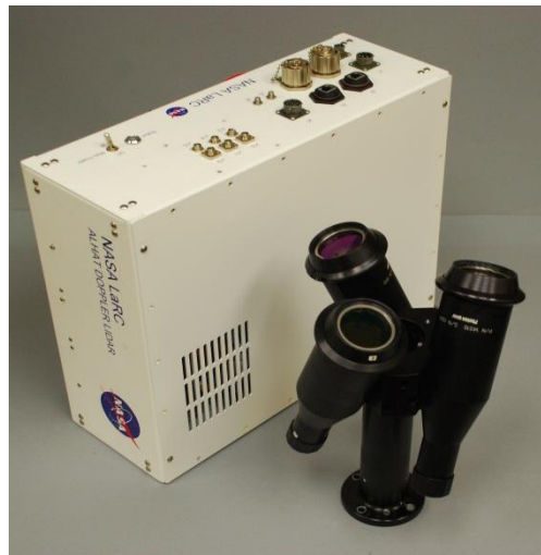
Figure 8. Prototype Doppler lidar system consisting of an electronic chassis and an optical head.
