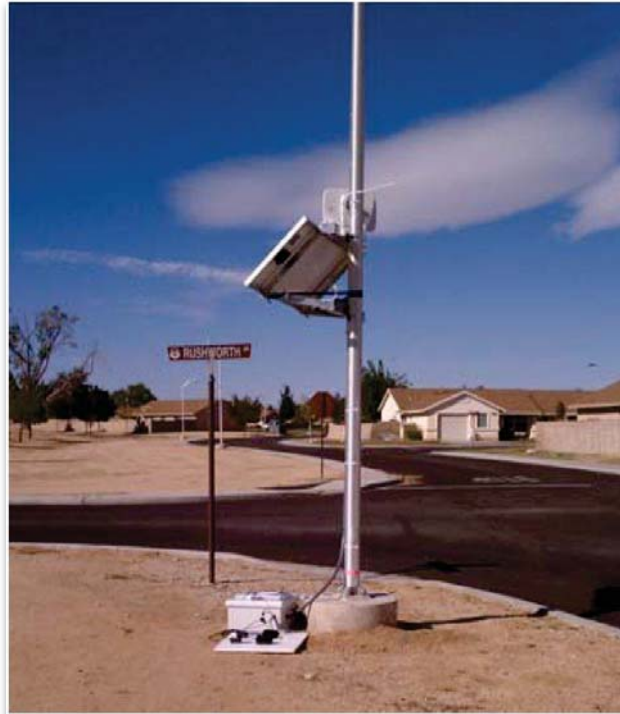
Figure 26. Sonic boom field kit installation photograph.
