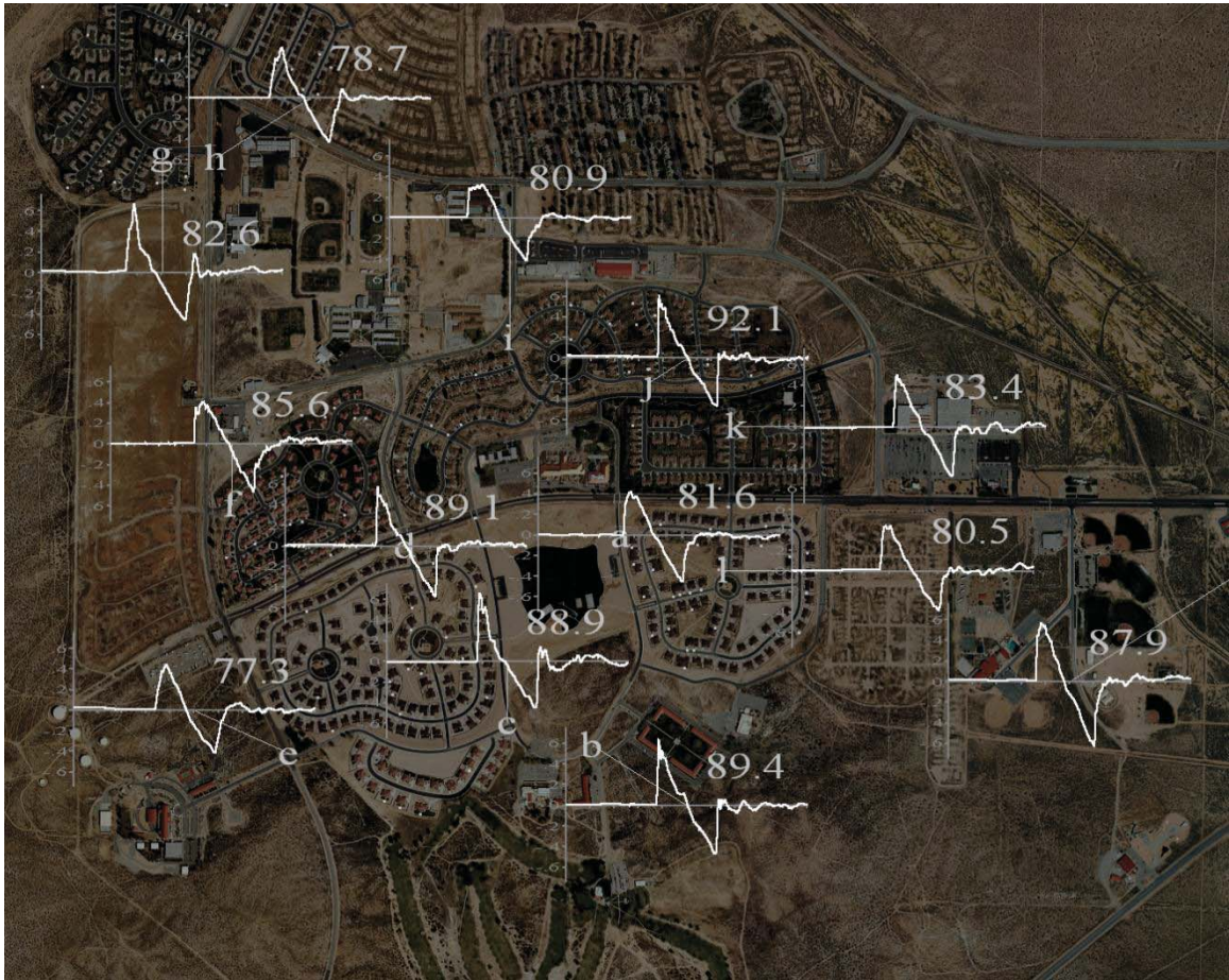
Figure 29. Measured sonic boom signature traces (psf) and Perceived Levels (PL) at monitor locations (a) full subject area including dormitories to the east and (b) close-up of the primary housing area.
