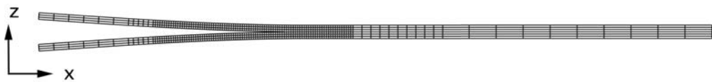
(a). Deformed model of a DCB specimen (plane strain CPE4 elements in Abaqus/Standard® and PLANE182 elements in ANSYS®) [7,8].
