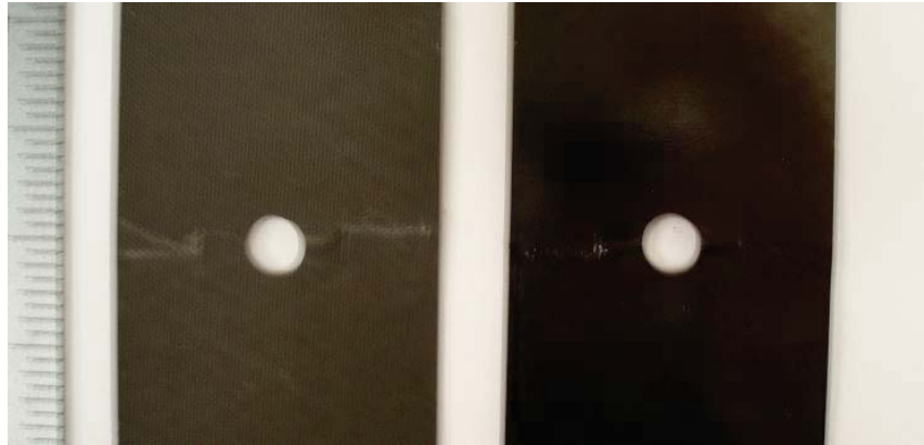
Figure 2. Image of representative OHC failure mode “LGM” in [60/-60/0]_S coupons, IM7/977-3 tested at RT-dry on the left and T40-800b/5320-1 tested at 177^\circ\text{C} -wet on the right.
