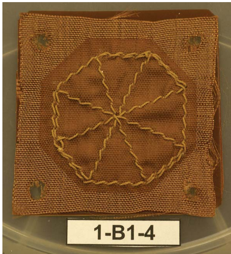
Figure 11. Triton TOR cloth and thread, MISSE-1 ram. Octagon is where sample was exposed to space.
