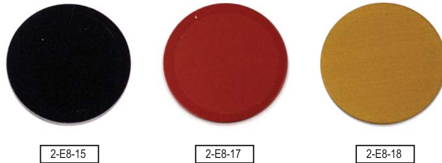
Figure 9. Postflight MISSE-2 dyed anodize samples.
