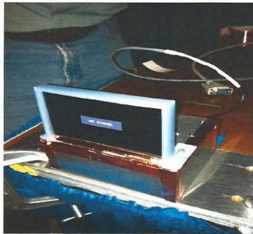
Figure 6 AMOLED #1 Mounted to the EMI Test Table
