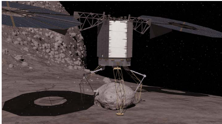
Figure 7. Hybrid Capture System Concept for the ARRM RBC Option (Image Credit: NASA/AMA, Inc.).
