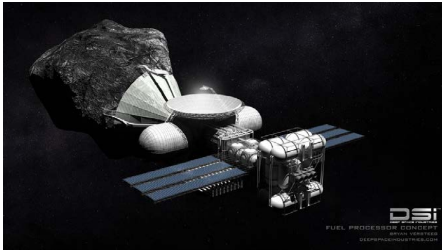
Figure 6. Asteroid Propellant Processing Concept (Image Credit: Bryan Versteeg / Deep Space Industries).
