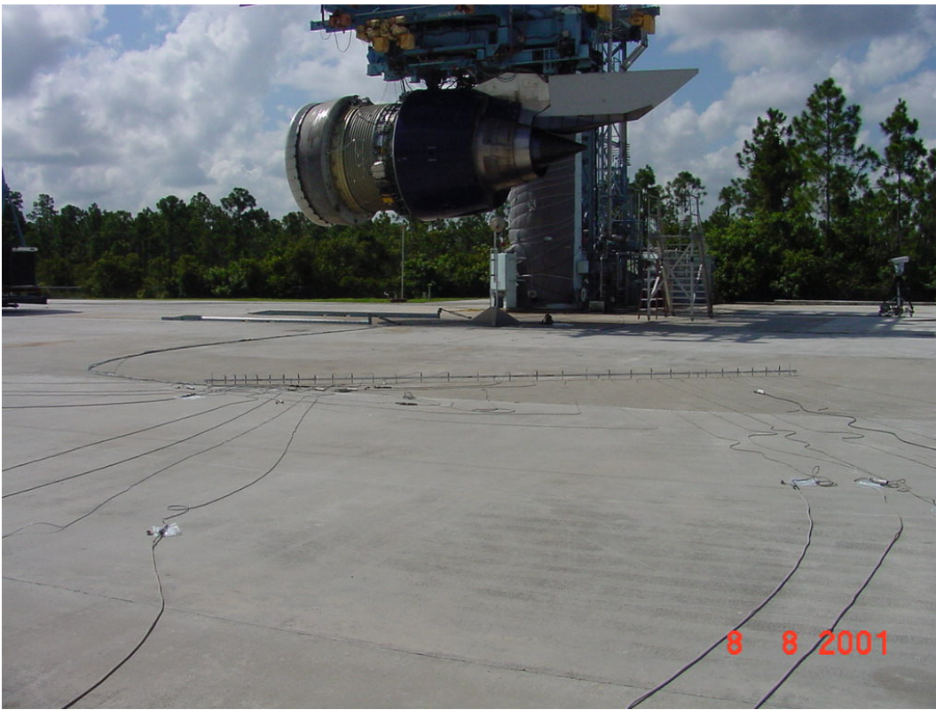
Figure 151.—Aft linear microphone array.
