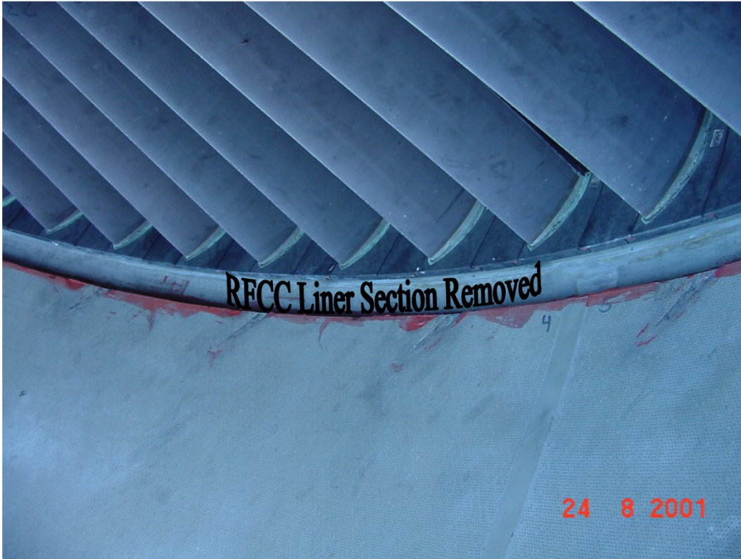
Figure 16.—Rear fan containment case (RFCC) liner section removed to accommodate 28 FEGV.
