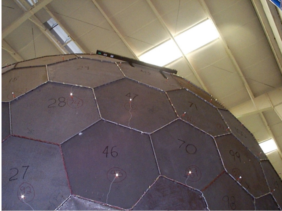
Figure 152.—ICD with phased array microphones installed.
