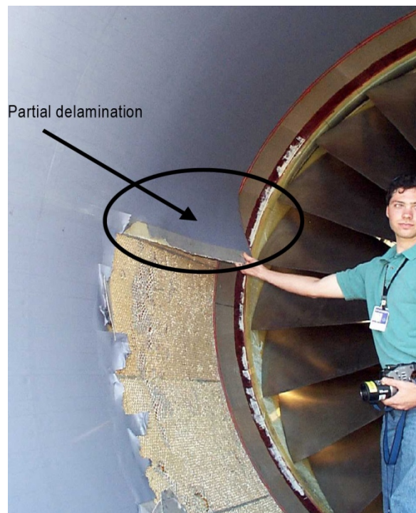
Figure 239.—Scarf inlet face sheet delamination—View 2.
