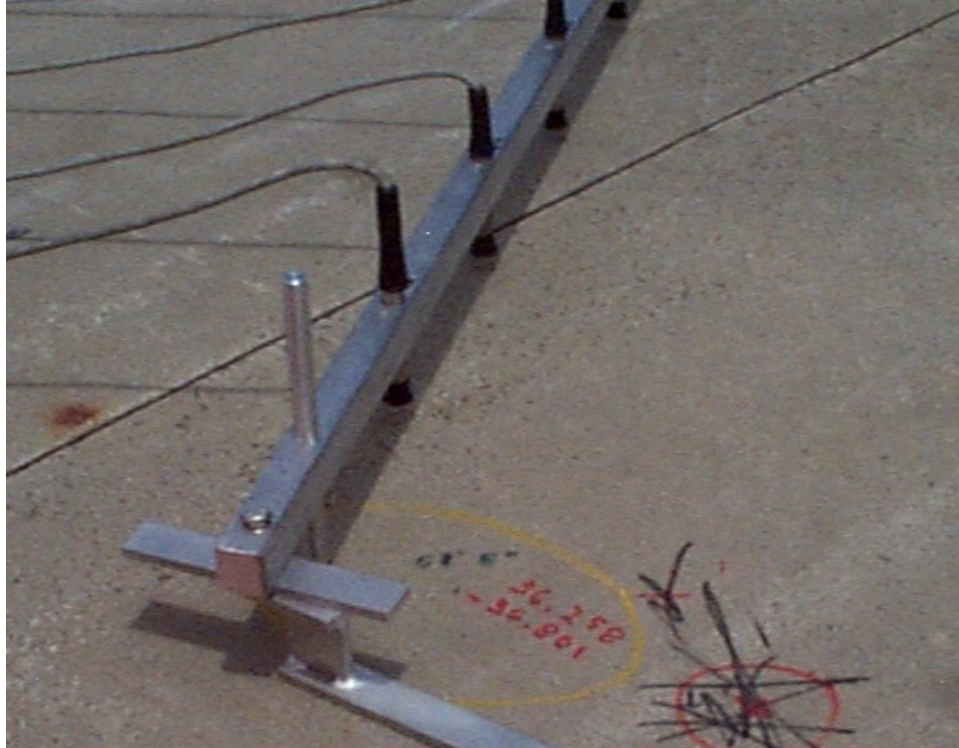
Figure 166.—Farfield linear array installation and locating pin.
