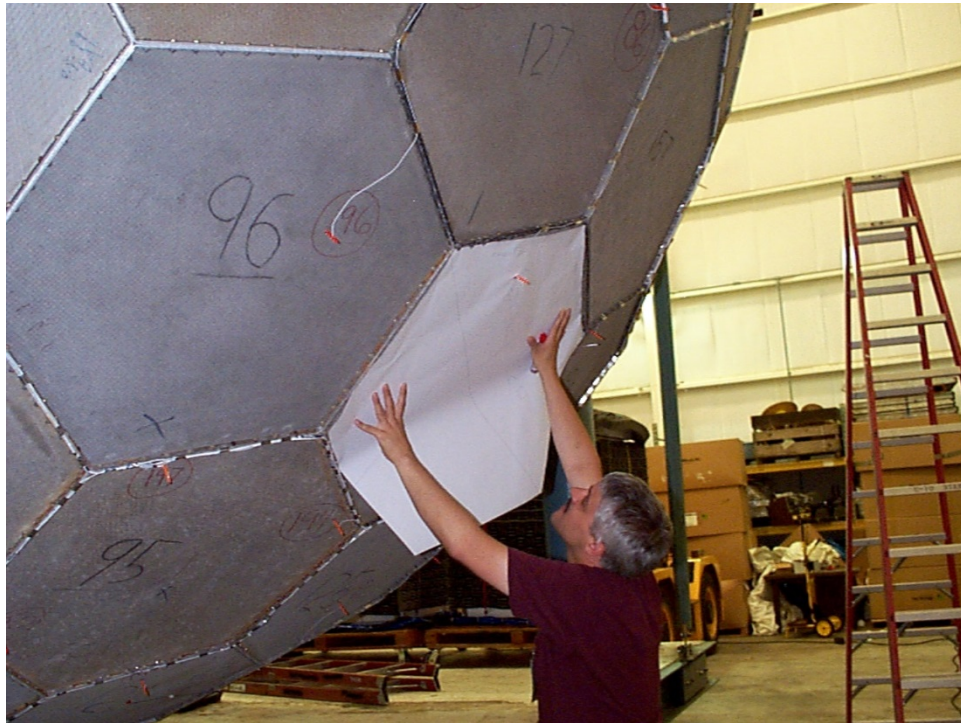
Figure 158.—Paper template for initial Kulite placement.
