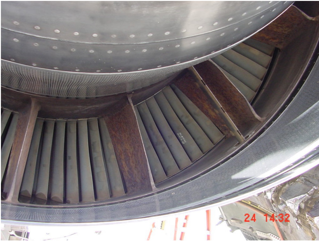
Figure 14.—Photo of tailpipe acoustic treatment.
