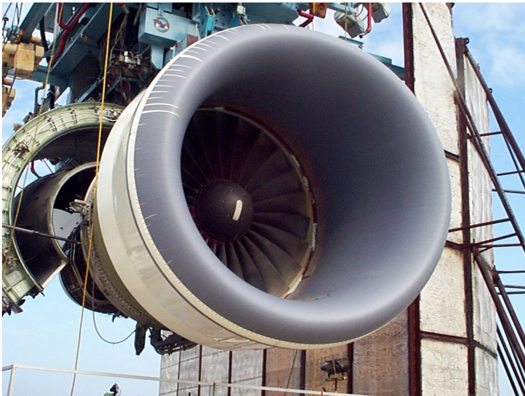
Figure 149.—Scarf inlet, taped hardwall, installed on PW4098 engine.
