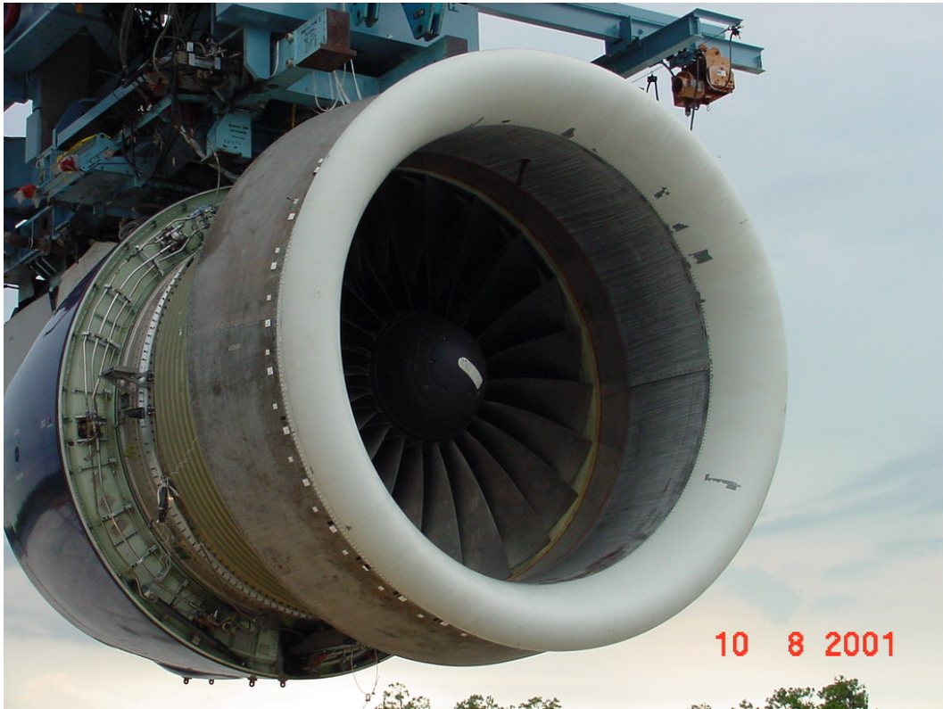
Figure 148.—Production inlet installed on PW4098 engine.
