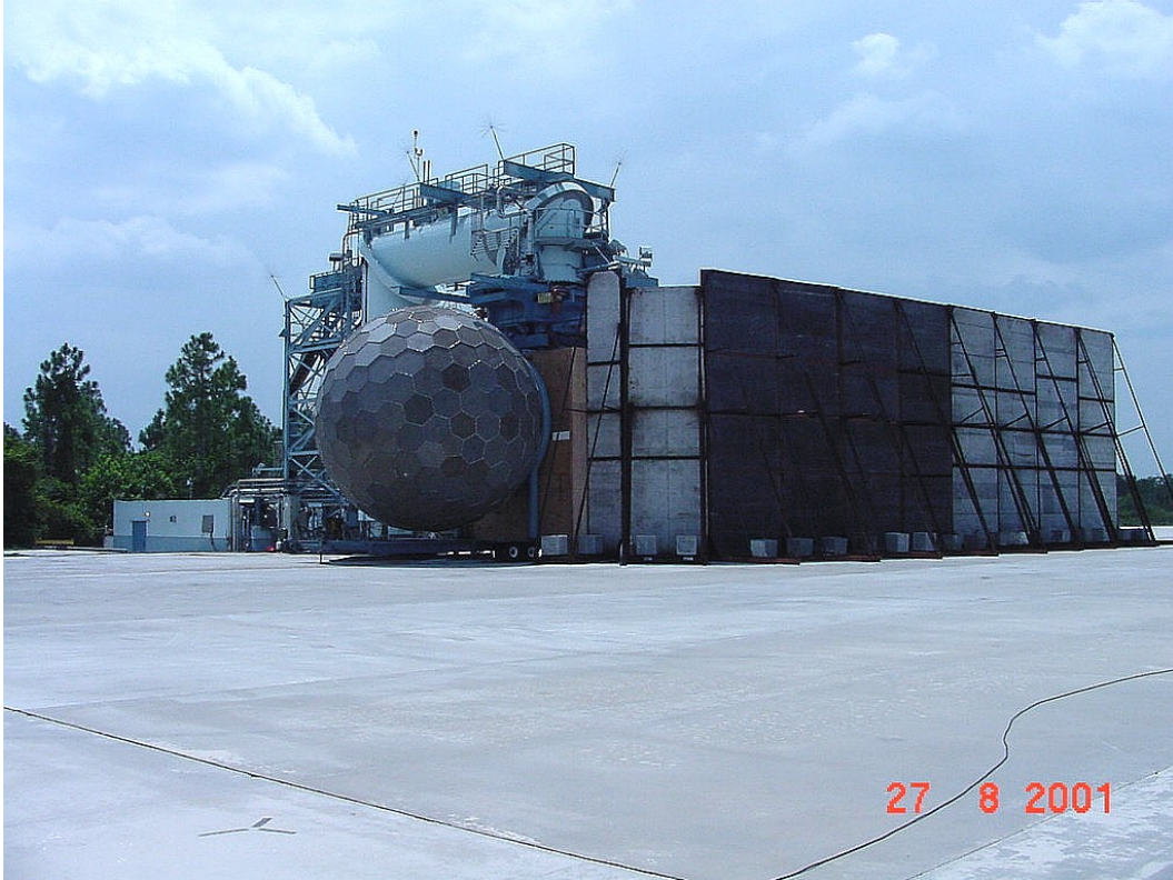
Figure 150.—Scarf inlet installed on PW4098 engine with ICD and aft barriers.
