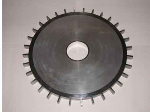
Figure 15.—Aluminum rotor disk with laser etched circular pattern.
