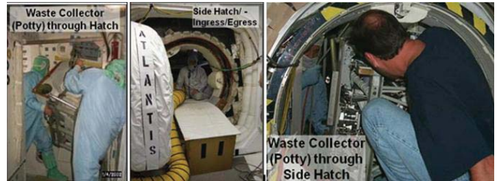
Figure 2 Hatch Ingress/Egress for Personnel/Hardware
