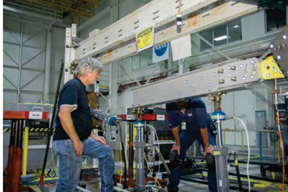
Figure 15. Pinning the hydraulic jacks to the load bar during a calibration testing preload setup.
