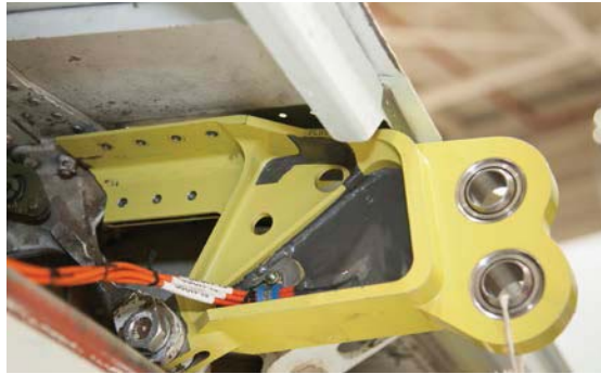
Figure 4. Closeup of an ACTE interface fitting attached to the left wing rear spar.
