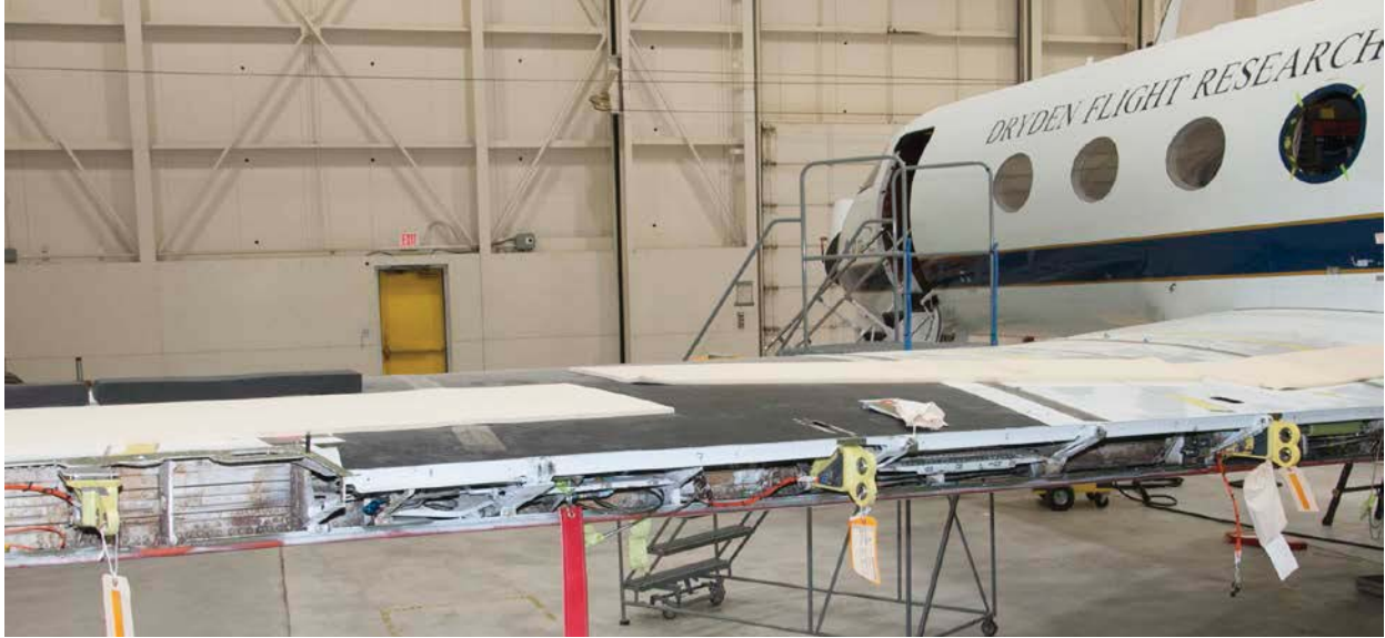
Figure 3. Three of four ACTE wing interface fittings attached to the left wing rear spar.
