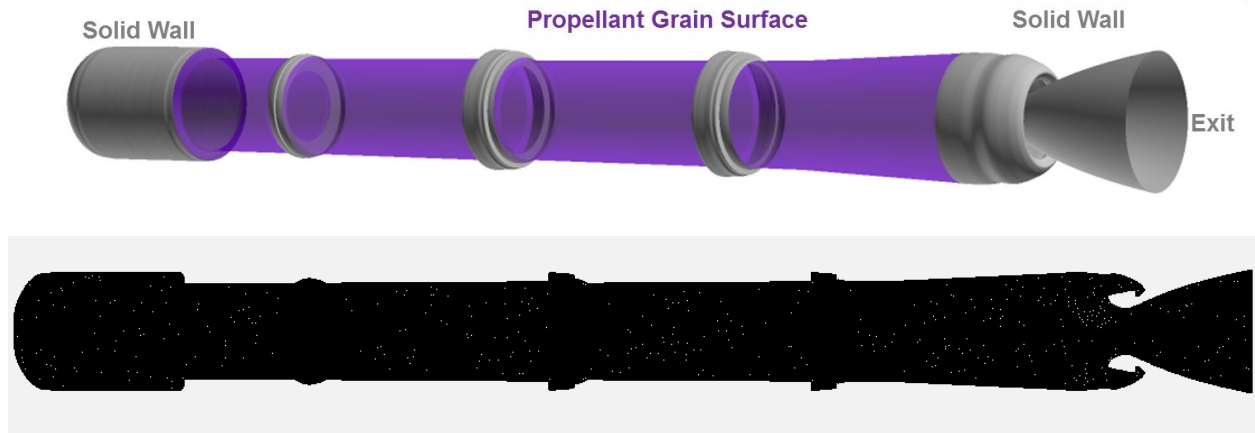
Figure 5. Geometry for reusable solid rocket motor (RSRM) problem: (Top) Illustration of propellant grain surface, solid wall, and exit boundaries; (Bottom) Cross-sectional cut of 3Dmesh.
