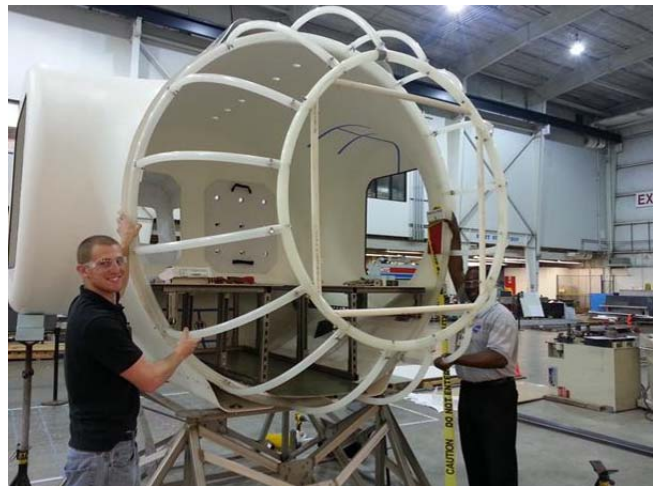
Figure 9. Low fidelity aft dome being fitted to underwater test mockup
