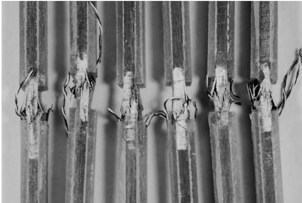
Figure 11. Edge-on view of unnotched compression specimens tested at 180°F
