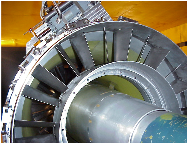
b) Close-up view of variable fan exit nozzle hardware arrangement
