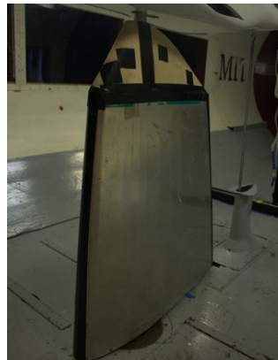
Figure 5: A photograph of the mounting hardware in the MIT Wright Brothers wind tunnel. (MIT)
