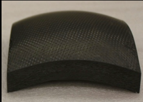
Post Arcjet Tested Coupons Resin Infiltrated
