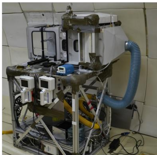
Figure 4: Test rig with full scale prototype installed in the Zero-G aircraft.
