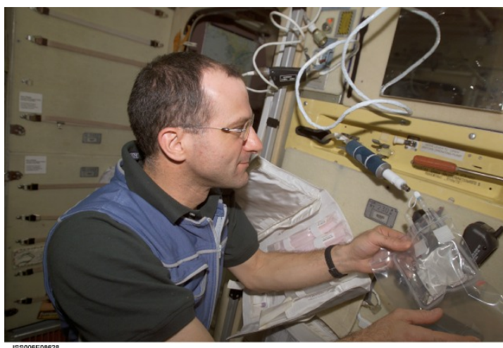
Figure 3. SVO-ZV Stored Water Dispenser Astronaut Donald Pettit collects a SVO-ZV sample.
