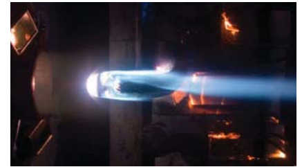
Teflon calibration test in the NASA Ames' Arc Jet Interaction Heating Facility.
