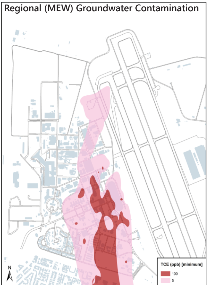
TCE concentration in the groundwater aquifer due to contamination from Regional (MEW) sources.
