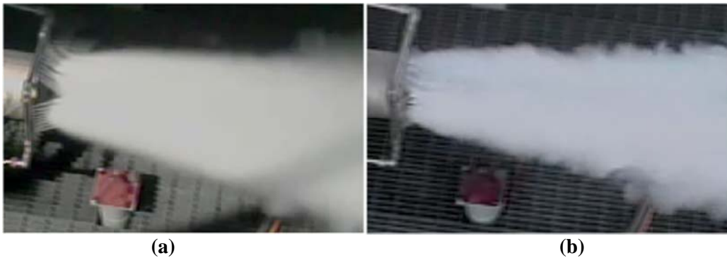
Figure 7: Flow Visualization of 1/8-inch Diameter Water Jet Injection (Qty. 32) at x/D_{DE}=-0.1 Upstream of SDT Exhaust Plane for Injection Angles of (a) 30^\circ and (b) 60^\circ
