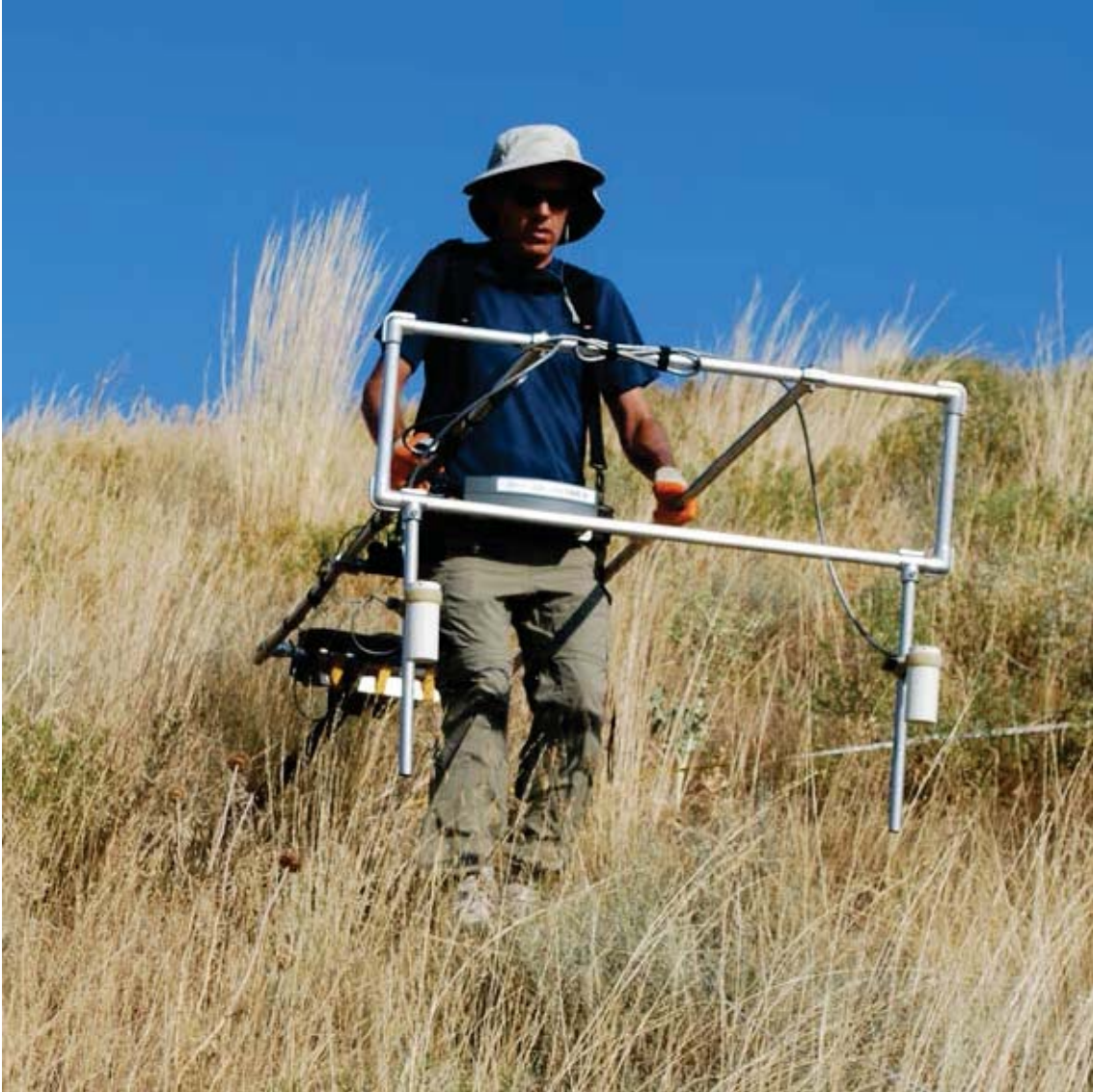
Figure 3A1. The NASA Team's 2-probe Geometrics model 858 magnetometer carried by Dr. Slayback on a Gordion tumulus. Dr. Slayback executed almost all of the magnetometer data collections and also processed the magnetometer data presented in this report.
