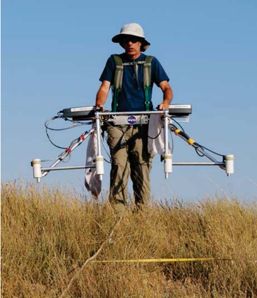
Appendix Figure 4.2. The NASA Team's 4-probe Geometrics model 858 magnetometers carried by Dr. Slayback on a Gordion tumulus. Dr. Slayback executed almost all of the magnetometer data collections and also processed the magnetometer data presented in this report.
