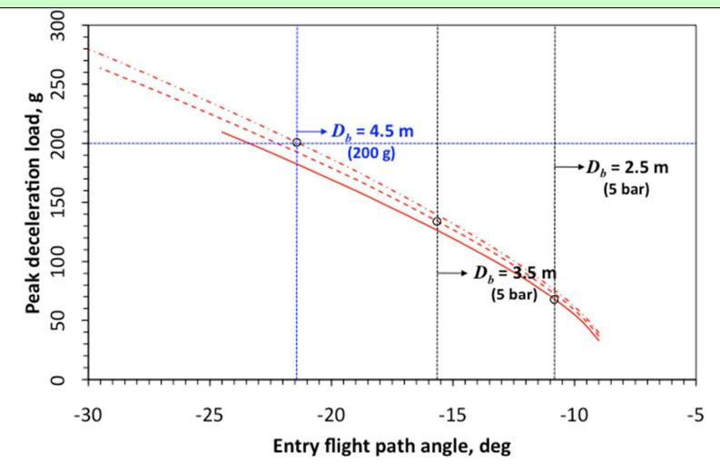
For 2.5 m and 3.5 dia., steepest entry is determined by the pressure limit (10 bar) For 4.5 m dia, steepest entry is still determined by g load limit
