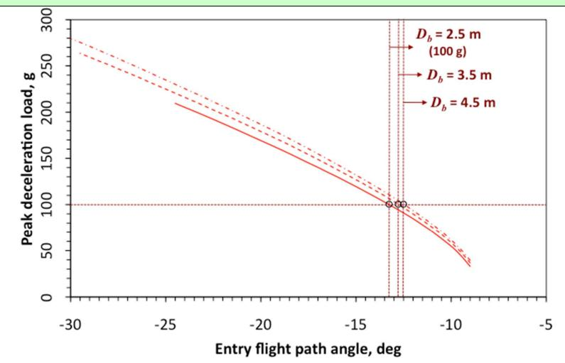
Steepest entry angle is determined solely by g load limit
