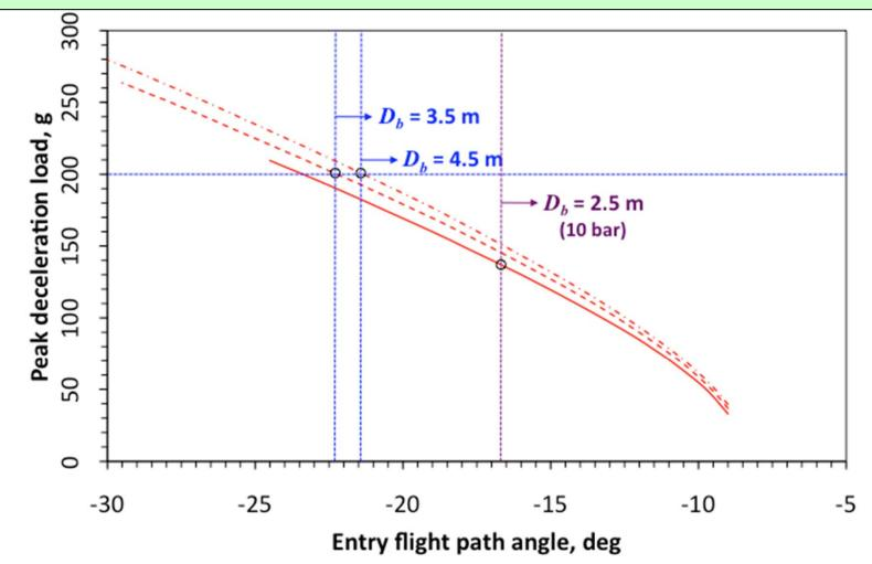
For 2.5 m dia., steepest entry is determined by the pressure limit (10 bar) For 3.5 m and 4.5 dia, steepest entry is determined by g load limit
