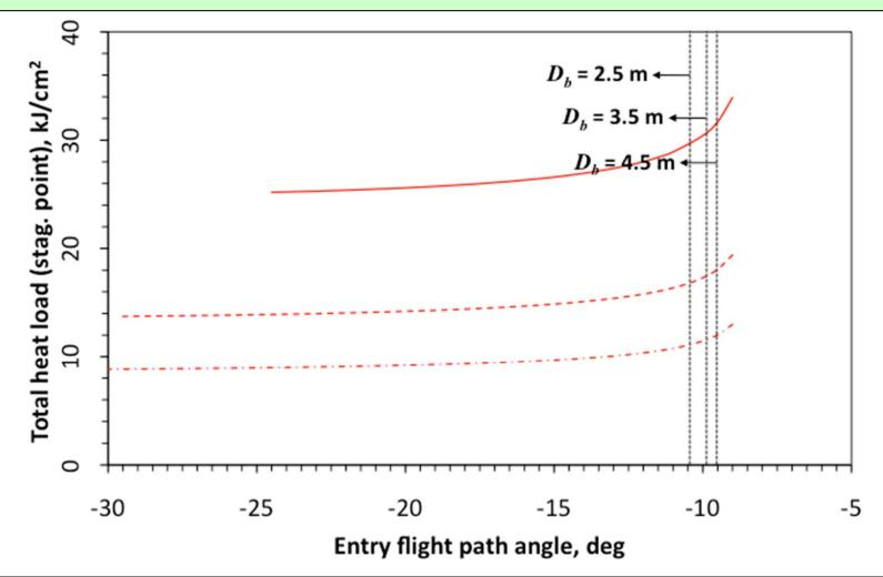
Entry angles correspond to max. curvature in heat load curves for highest  $\beta_E$ These entry angles close the entry flight path angle interval at the shallow end
