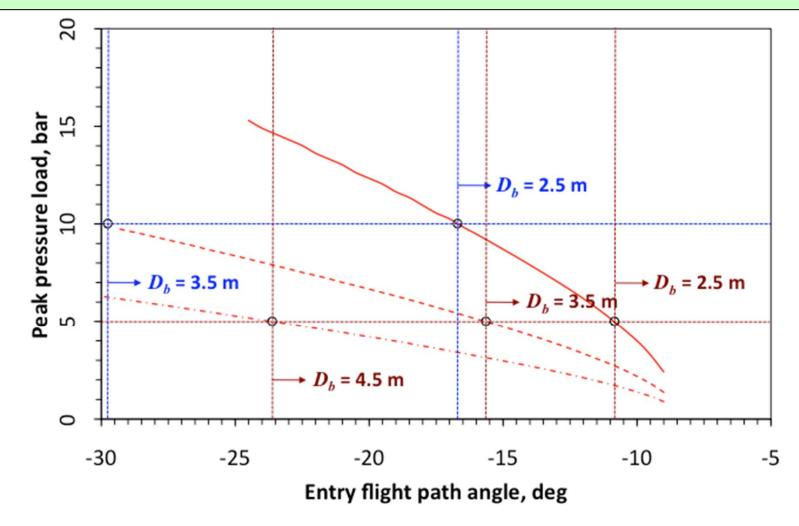
Are the deceleration load and pressure load constraints mutually exclusive? The answer is, "Yes. For some ballistic coefficients, pressure is the key"
