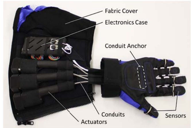
Fig. 2. Forearm Layout, Conduit Anchor, and Sensors
