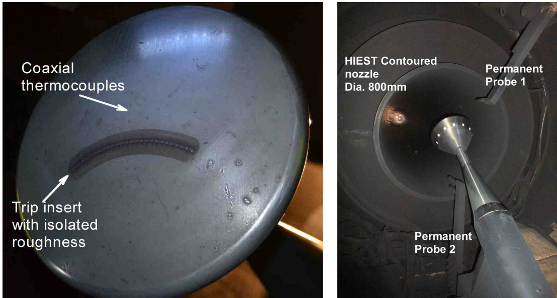
Fig.4 Left: Heat shield surface of Apollo CM test model with ‘pizza-box’ shaped isolated roughness elements ( k=0.3\text{mm} ) on a trip insert. Right: Photo of Apollo CM test model installed in the HIEST test section.
