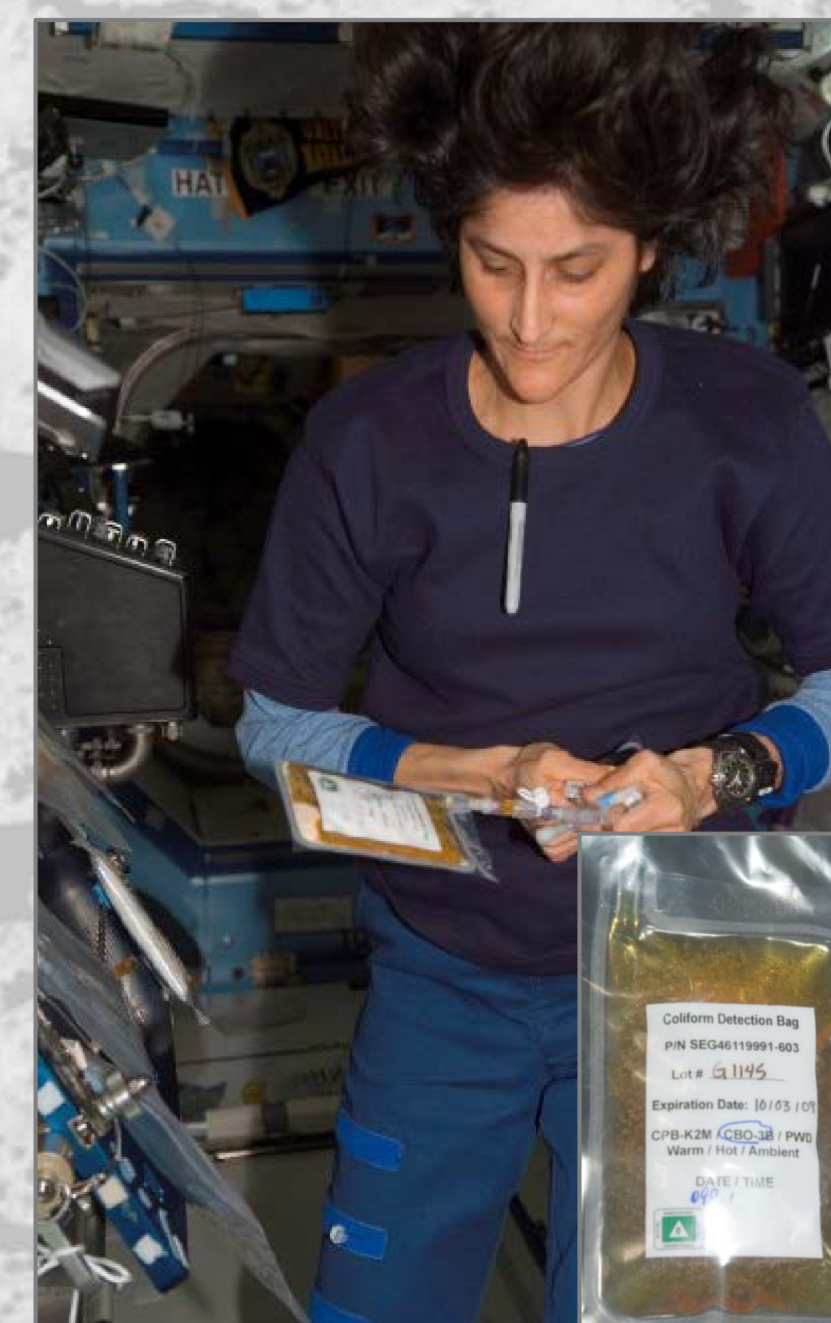
The Coliform Detection Packet is used to detect E. coli and coliforms in potable water on ISS.
