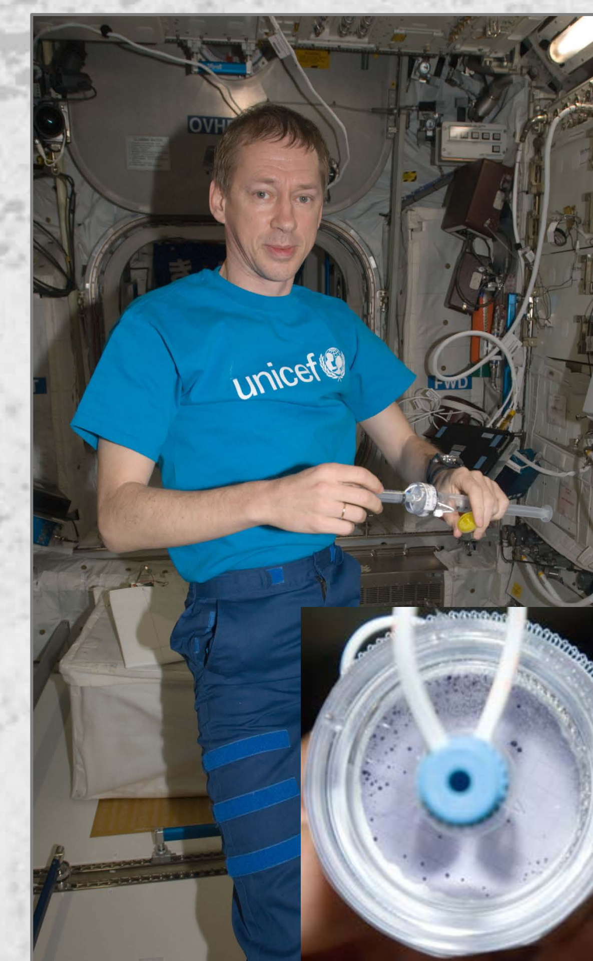
The Microbial Capture Device is used to enumerate heterotrophic bacteria in potable water on ISS.
