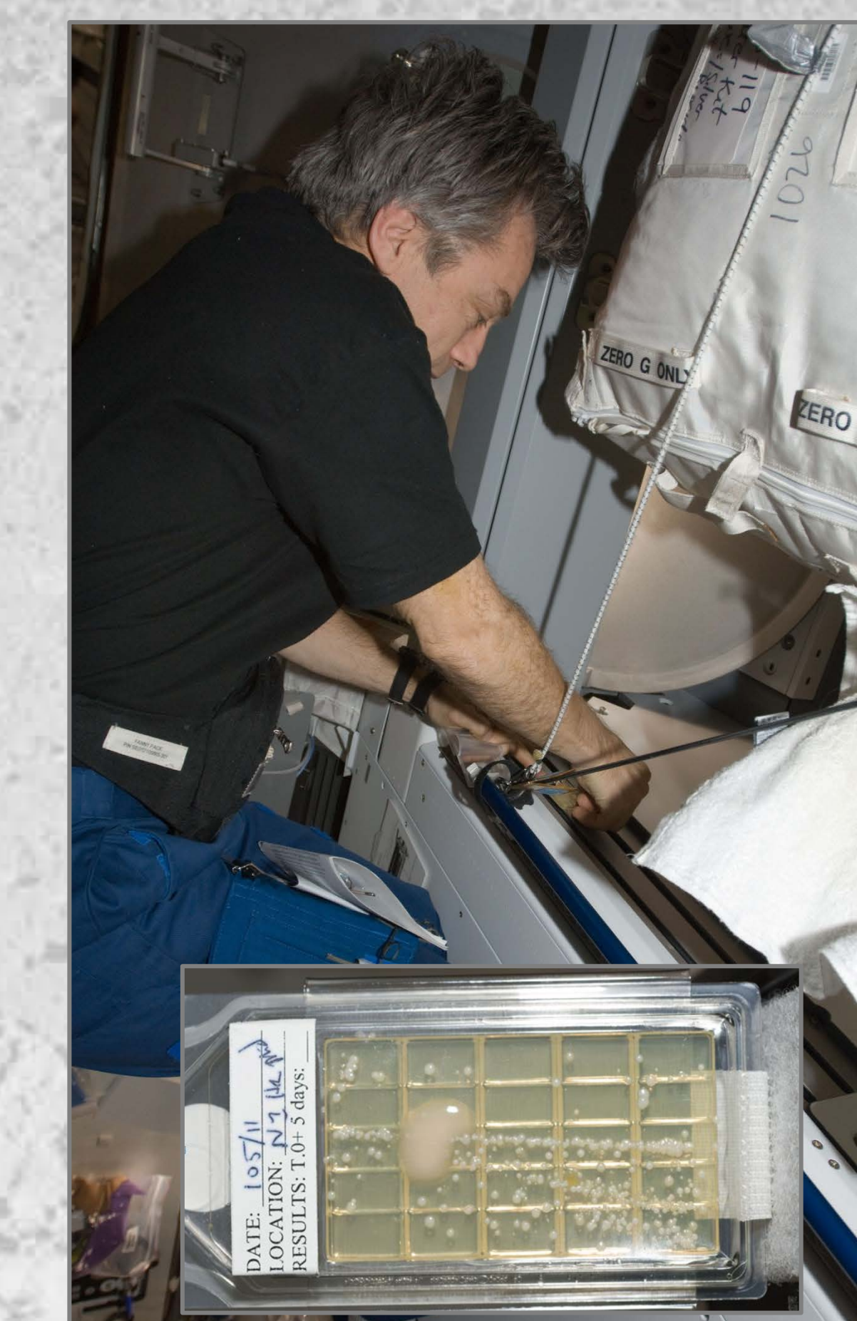
The Microbiology Surface Sampling Kit (SSK) is used to enumerate bacteria and fungi on ISS surfaces.
