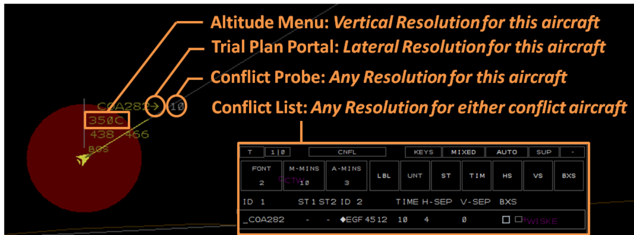
Figure 2. Points of access available to invoke the auto resolver and associated resolution preferences.
