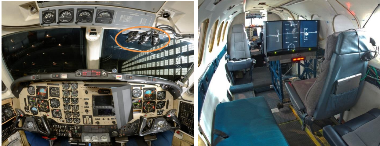
Figure 7. XVS Cameras and Display Installation
