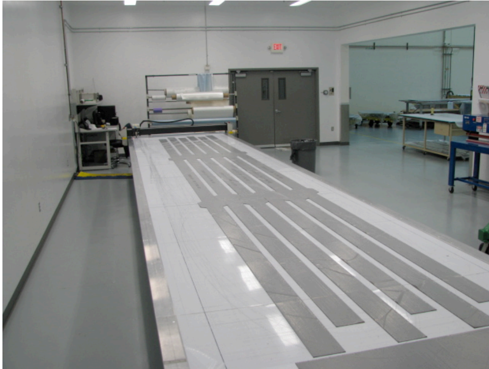
Figure 3. Nested Flat Patterns for Stringer Preforms CNC Cut from Multi-Axial Carbon Fiber Fabric
