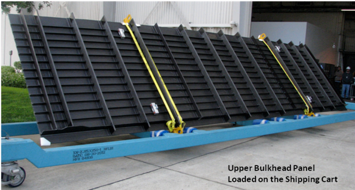
Figure 92. Upper Bulkhead Loaded on the Shipping Cart
