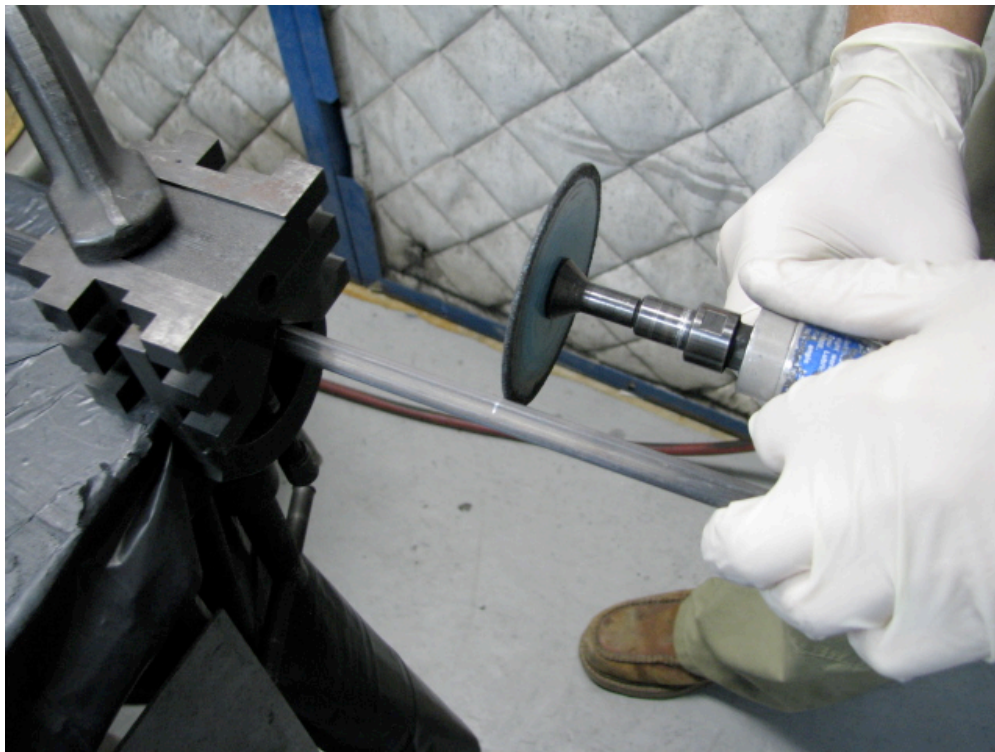
Figure 11. Rough Cutting of a Pultruded Carbon Fiber Epoxy Rod to Length
