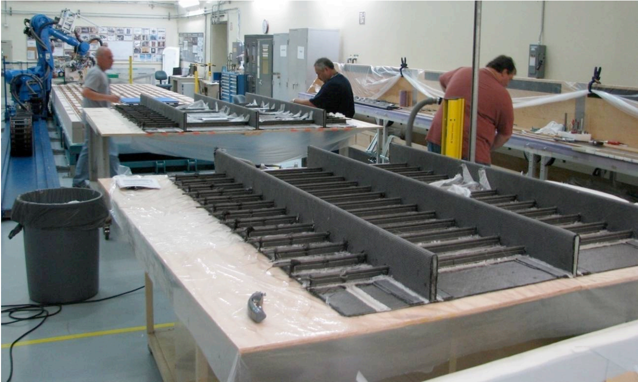
Figure 70. Two Outer Rib Preforms were Fabricated Simultaneously
