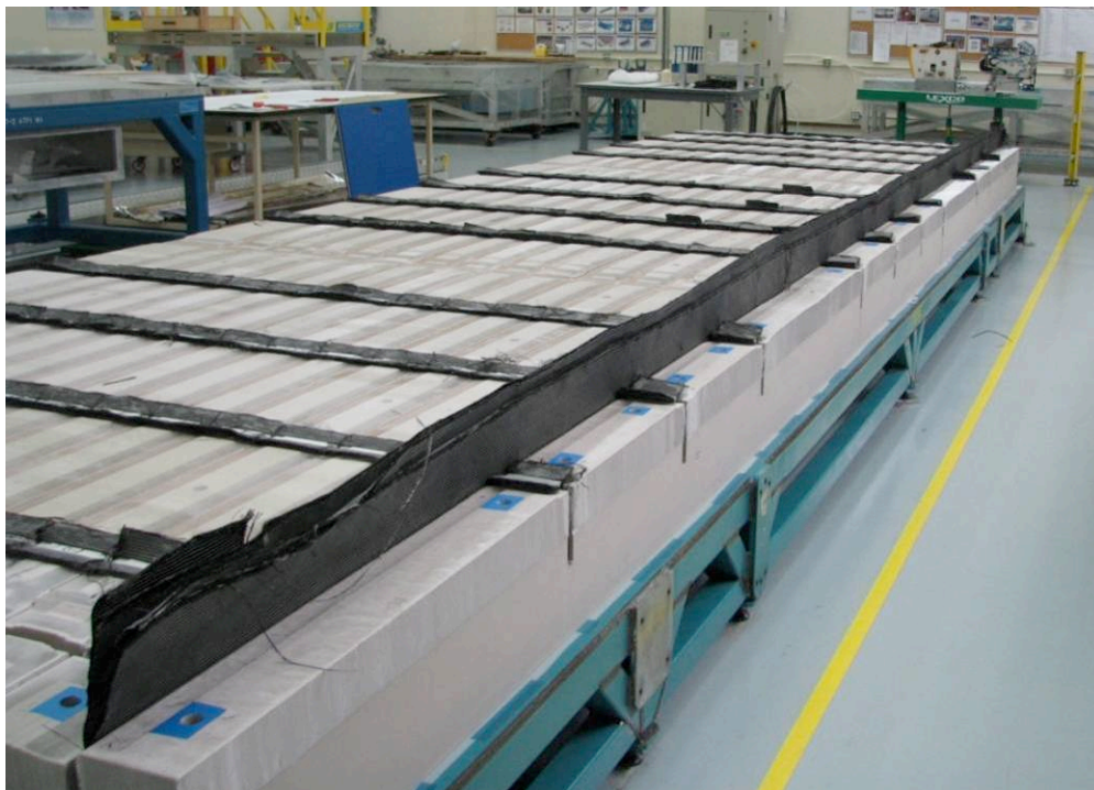
Figure 80. Integral Cap Stacks at Panel Floor Line Installed
