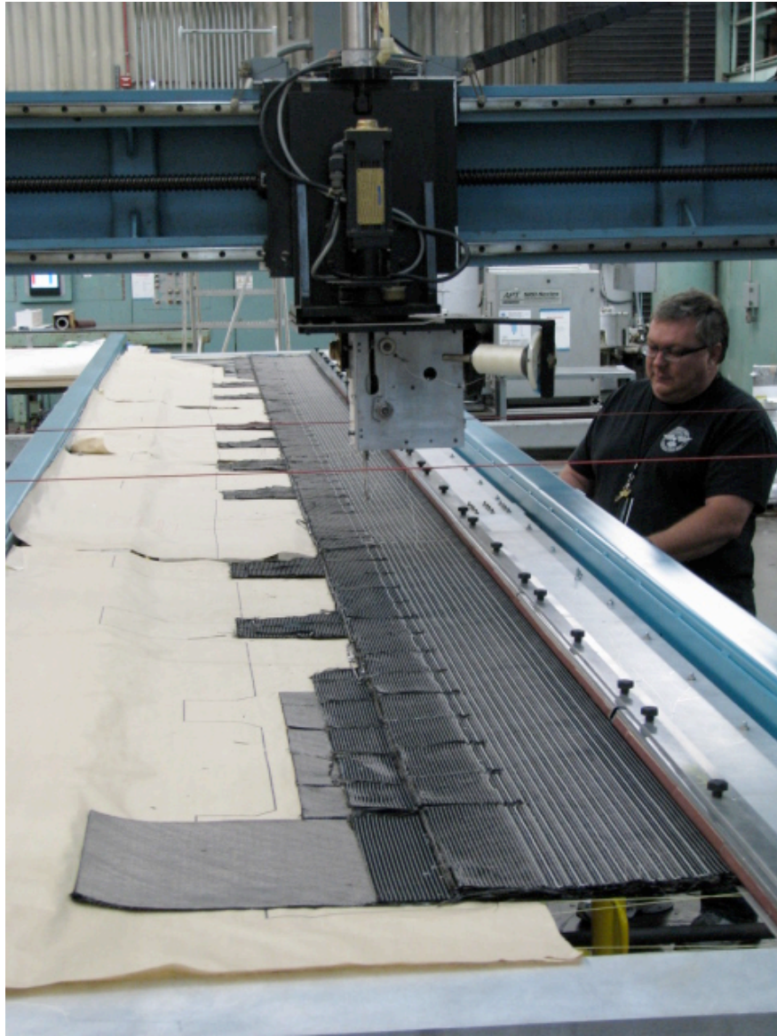
Figure 10. Stitching of Crown Panel Cap Web on the Gantry Sewing Machine
