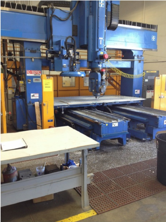
Figure 98. Drill Template was Fabricated to Drill DA Holes on the Panels
