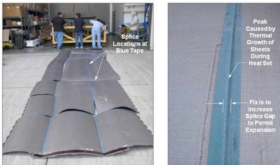
Figure 42. Perforated Caul Sheets from Crown Panel Infusion (Revised for Subsequent Panels)
