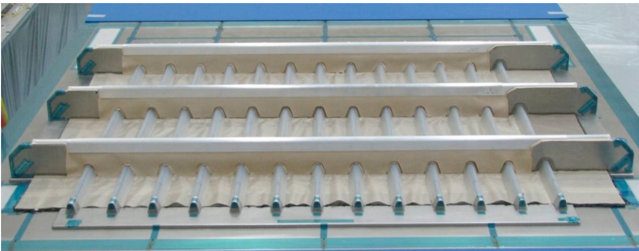
Figure 71. IML Tooling Placed on Preform
