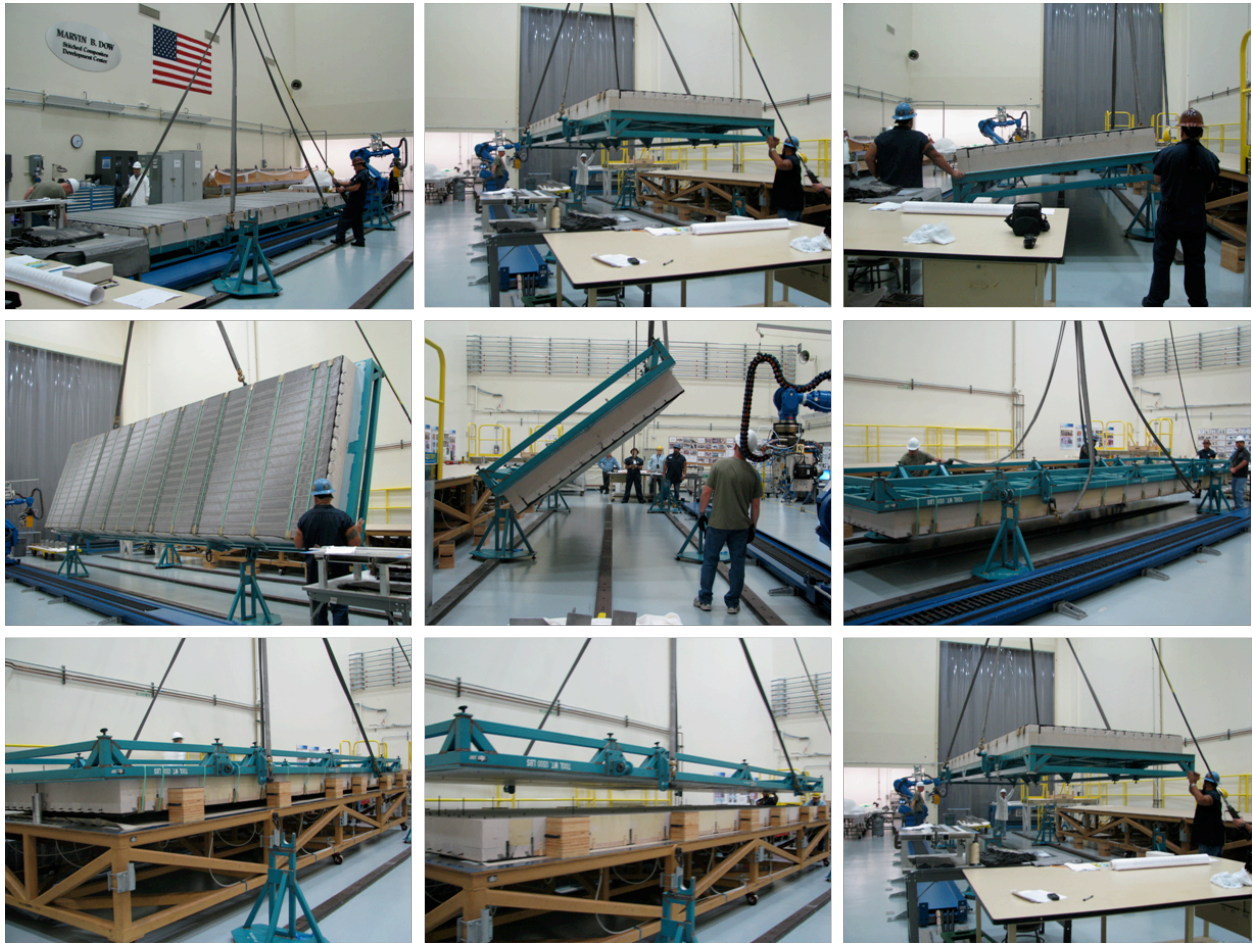
Figure 88. Transferring the Upper Bulkhead Panel Preform onto the Cure Tool
