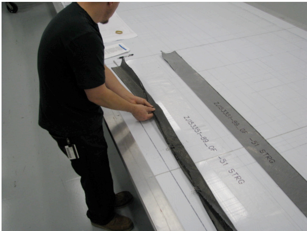
Figure 5. Stringer Flat Pattern Folded Over Leader Wire
