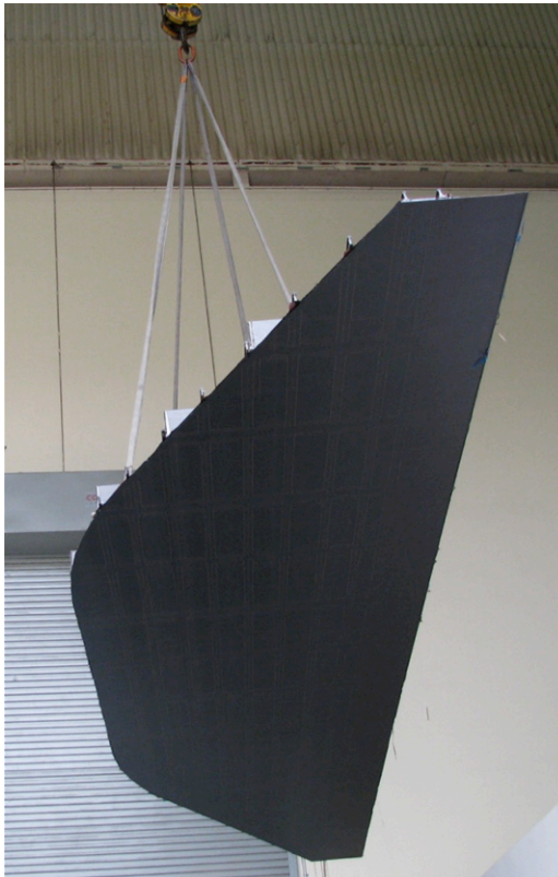
Figure 108. OML and IML Surfaces of the Cured Lower Bulkhead Panel Prior to Trimming
