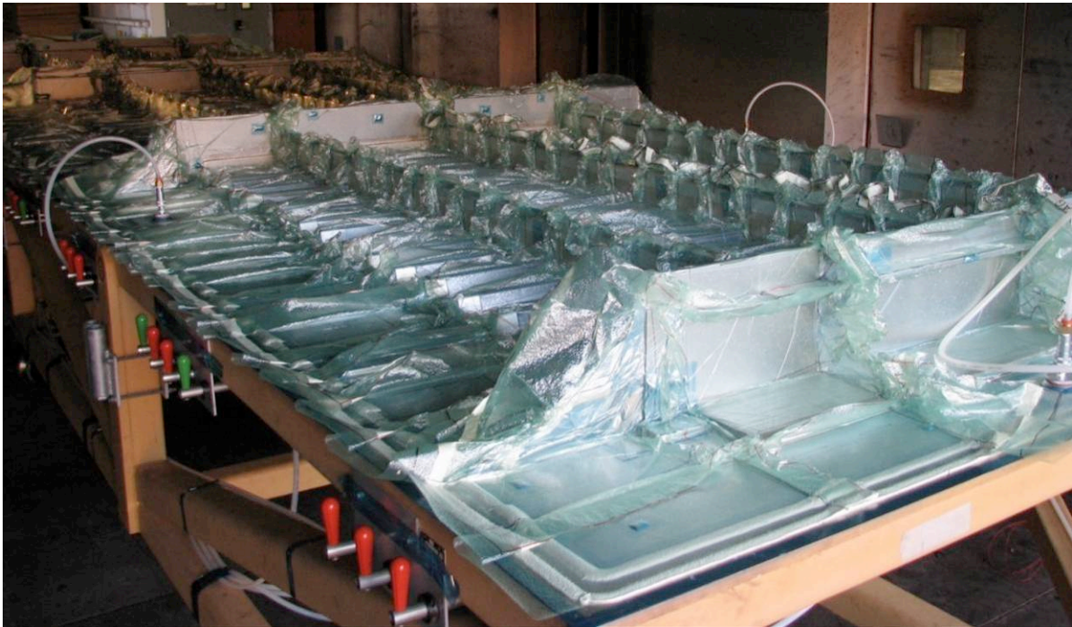
Figure 63. Floor Panel Preform Placed in Oven Ready for Heat-up, Infusion, and Cure
