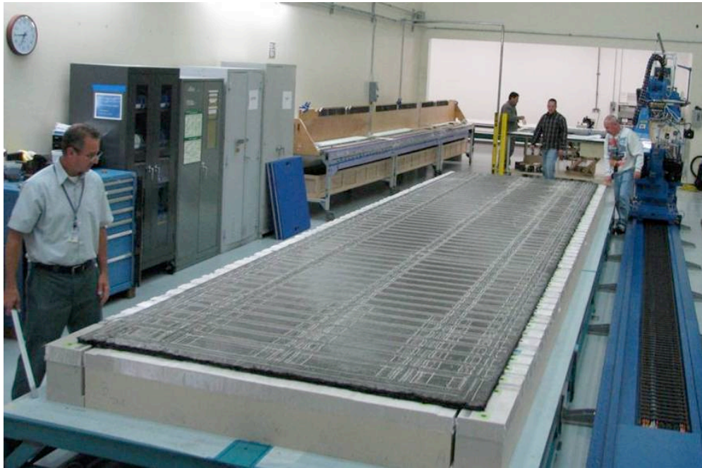
Figure 26. Completed Crown Panel Preform Stitching
