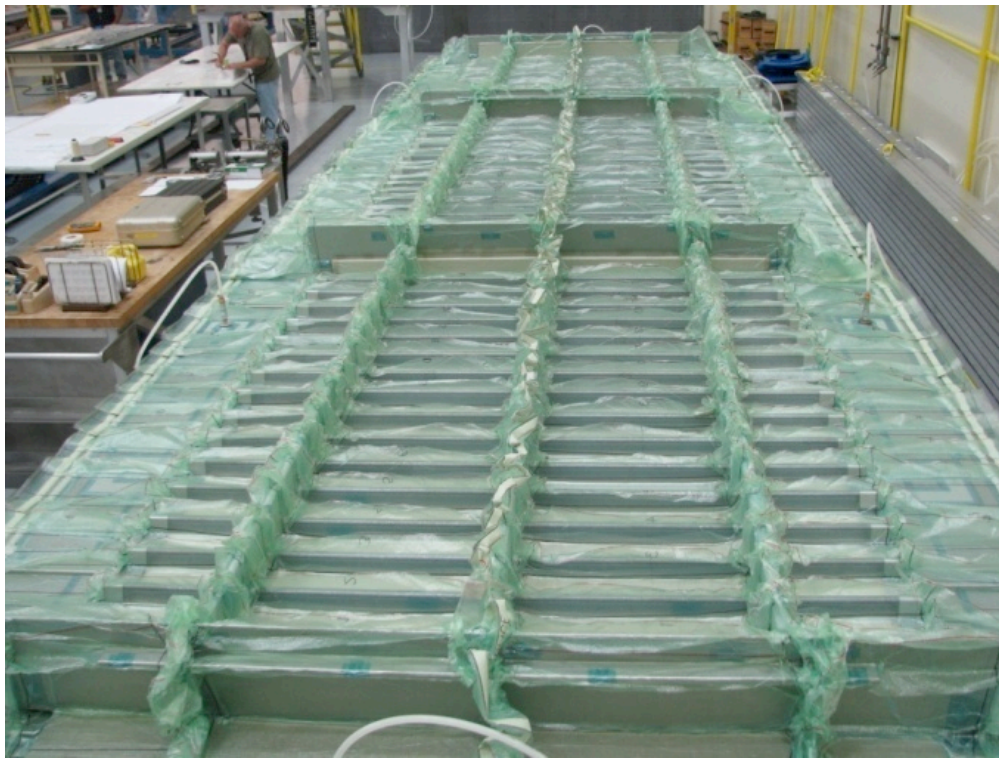
Figure 62. Secondary Bag Installed and Leak Checked
