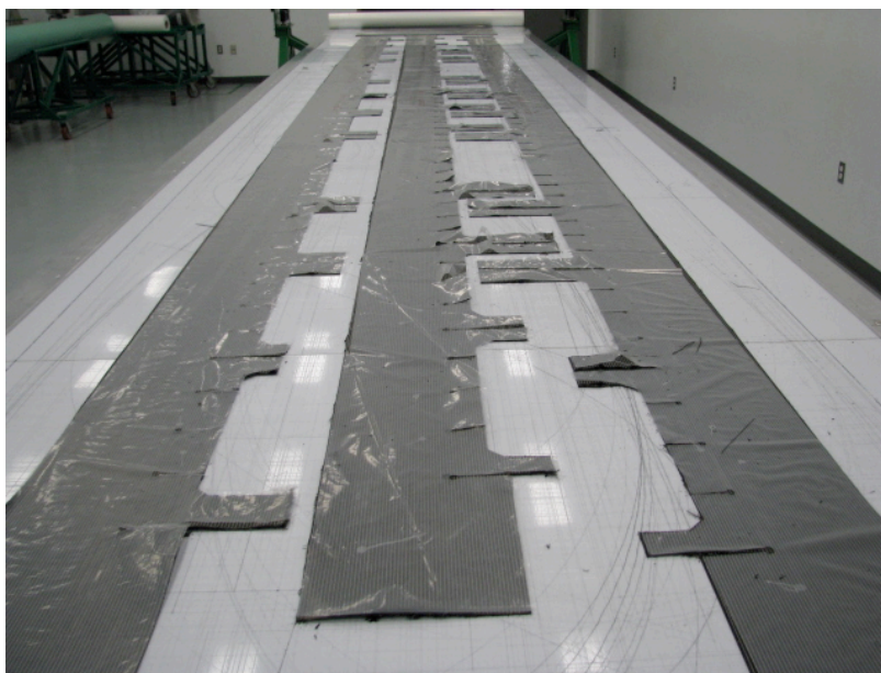
Figure 9. Nested Flat Patterns for Crown Panel Cap Preform
