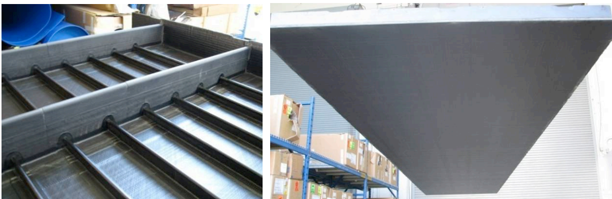
Figure 66. Floor Panel IML and OML Cured Part Surfaces
