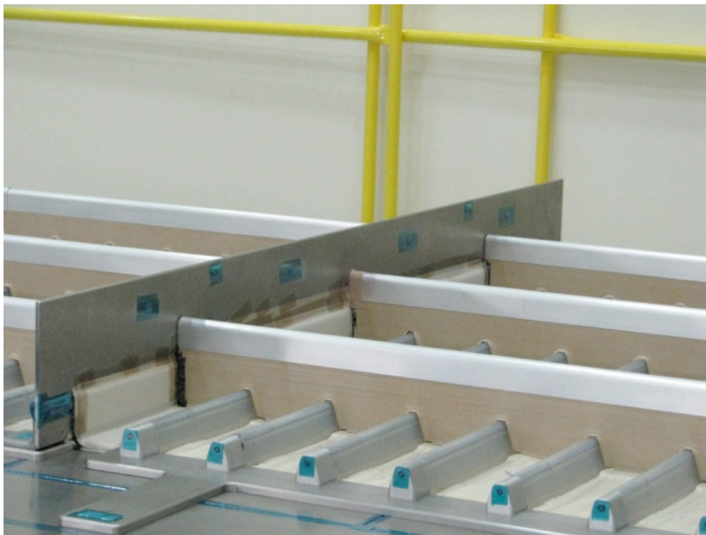
Figure 57. Bagging Aids on Frames and Stringers
