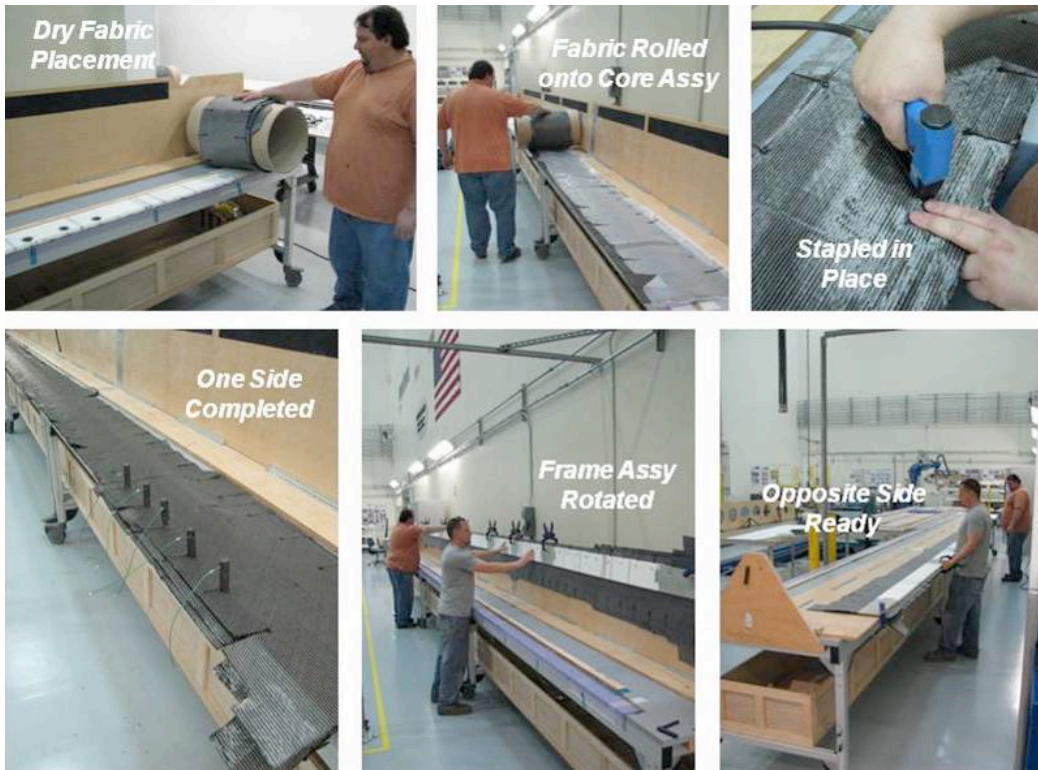
Figure 20. Wooden Assembly Tool Used to Attach Fabric to Foam Core
