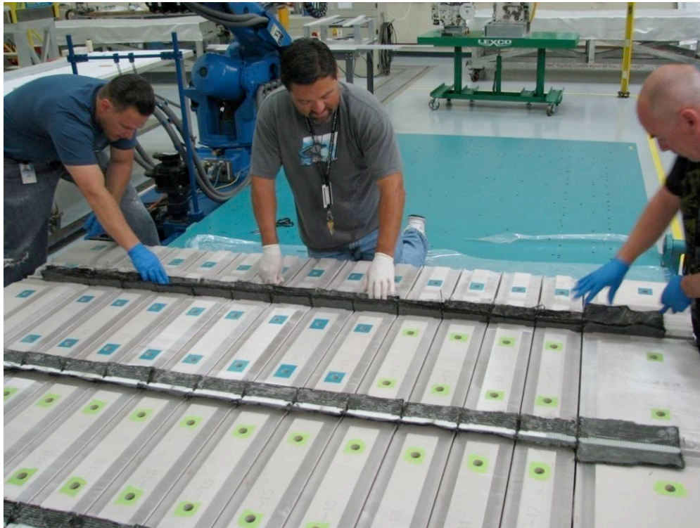
Figure 67. Outer Rib Preform Assembly – Frame Installation
