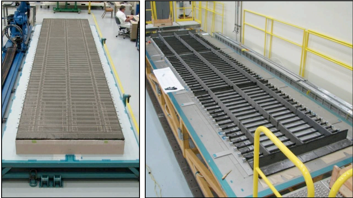
Figure 55. Completed Floor Panel Stitched Preform
