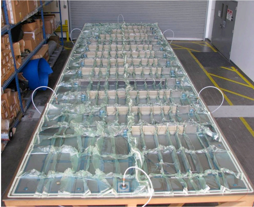
Figure 107. Vacuum Bagging Complete Ready for Transporting the Assembly to the Oven
