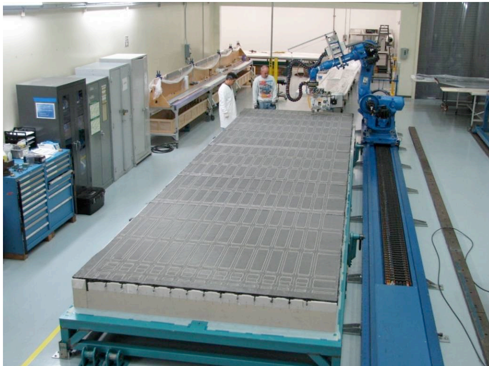
Figure 87. First Upper Bulkhead Panel Stitching Completed
