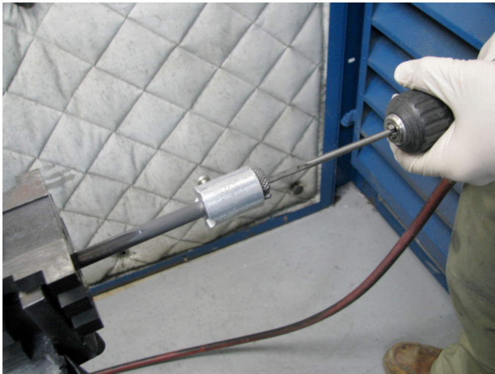
Figure 13. Drilling of Rod End to Accept Nylon Set Screw for Mounting of Leader Wire Adapter
