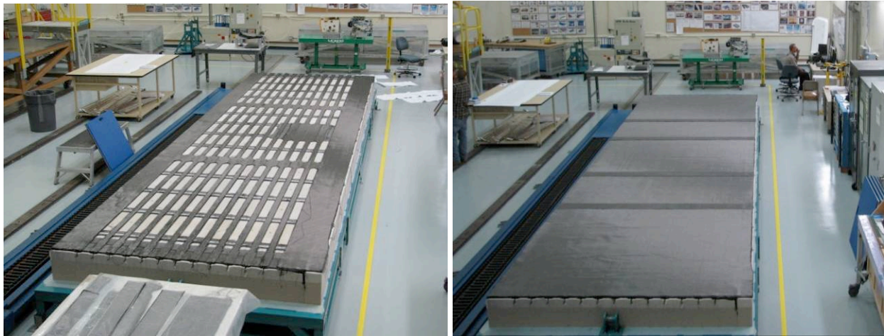
Figure 86. Tear Straps Placed First, Followed by Skins and Skin Stack Splices
