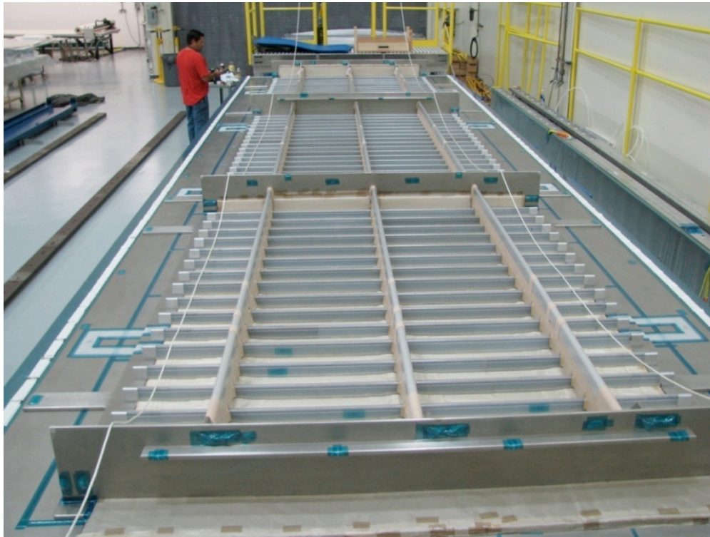
Figure 59. Added Lanyards to Support Bag During Unrolling Operation
