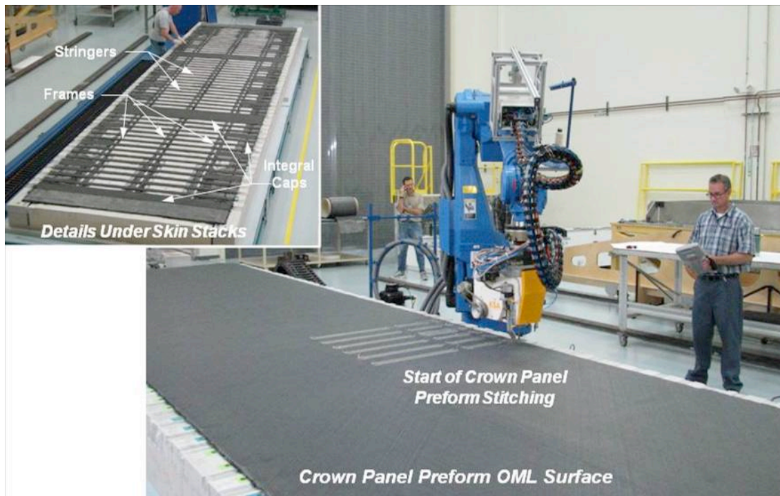
Figure 25. Single-Sided Stitching of Crown Panel Preform Started
