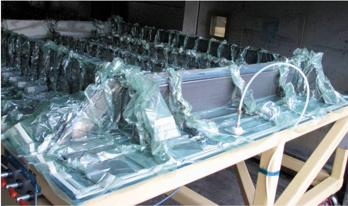
Figure 37. Infusion and Initial Cure Completed
