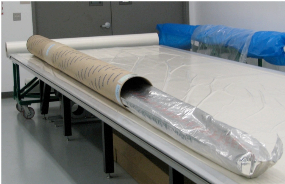
Figure 58. New Pre-Conditioned Vacuum Bag Delivery Packaging
