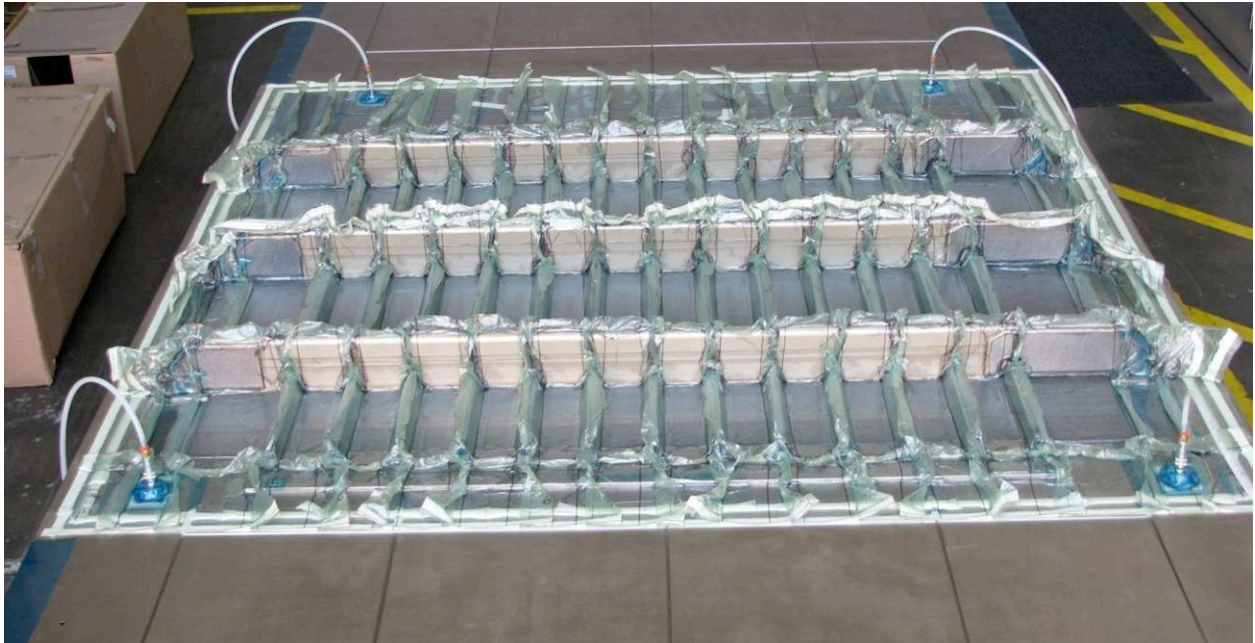
Figure 72. Bagged Outer Rib Panel During Vacuum Check
