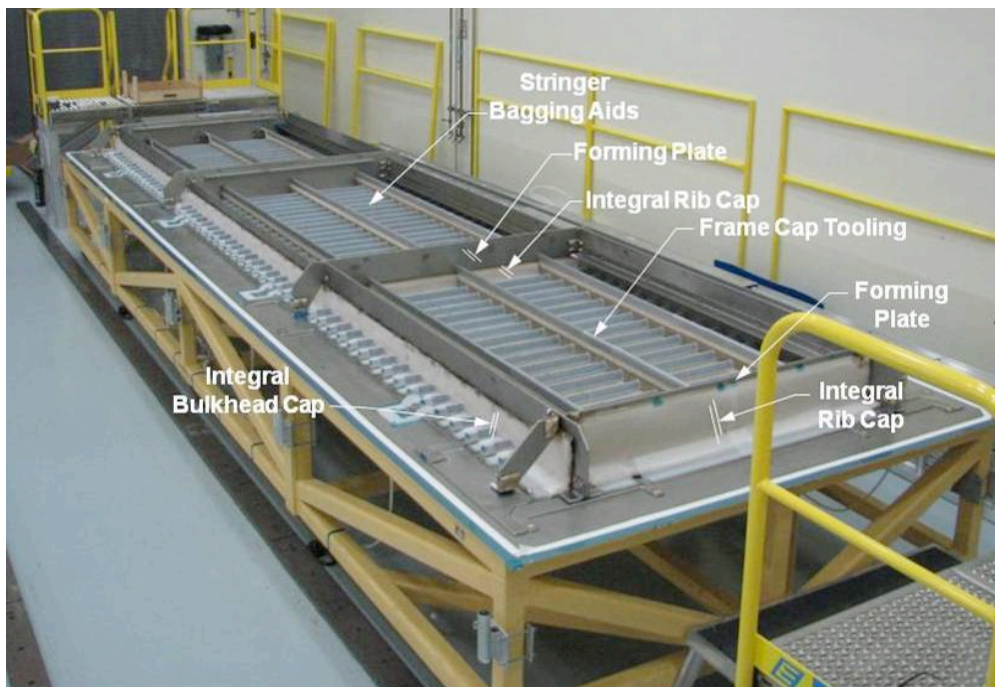
Figure 32. Under Bag IML Tool Details Located
