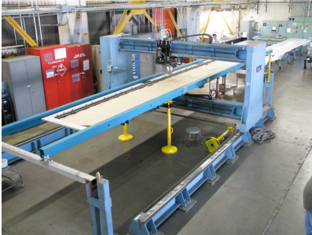
Figure 6. Stringer Preform on Gantry Style Sewing Machine
