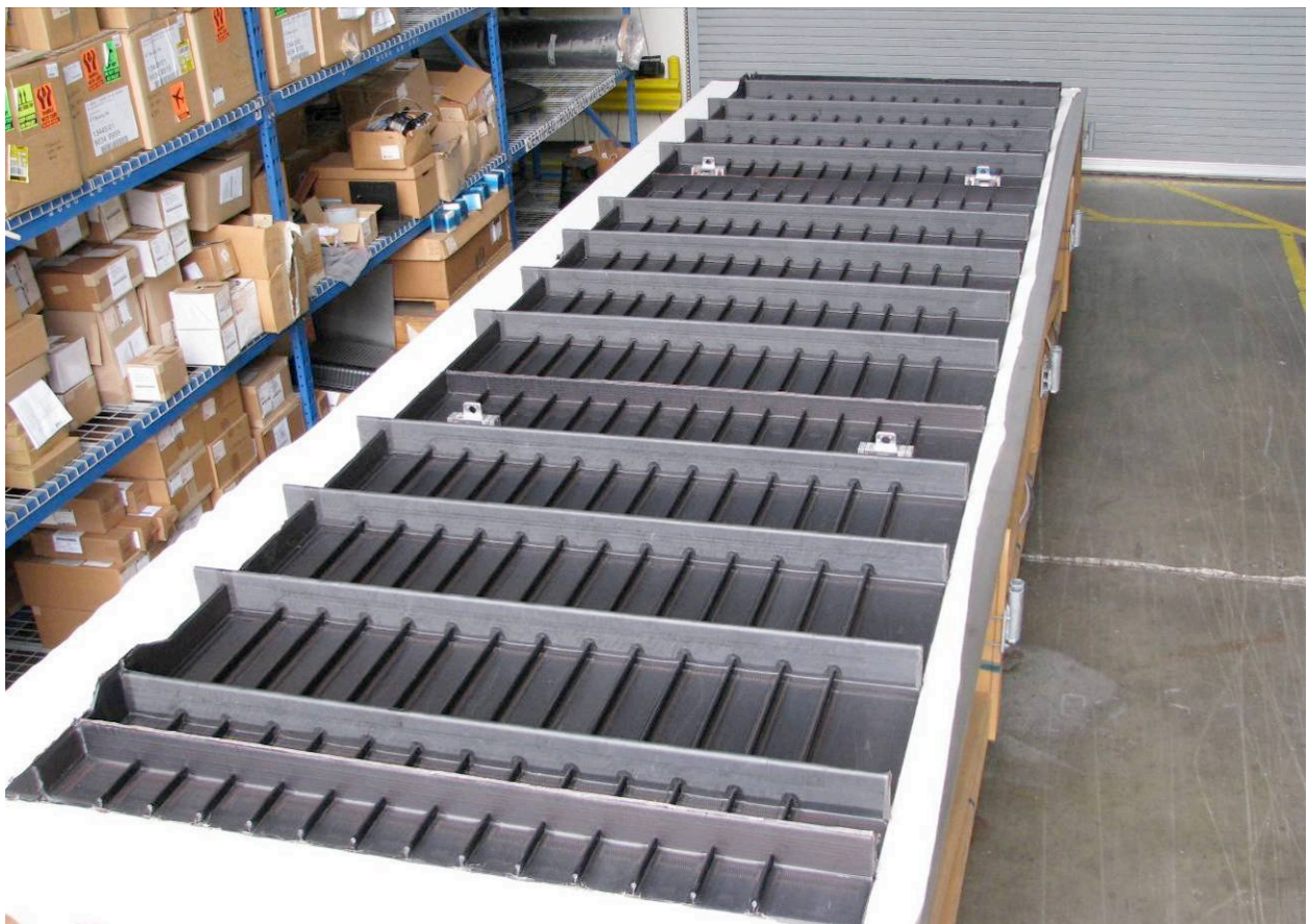
Figure 91. Cured Upper Bulkhead Panel Ready for Trim
