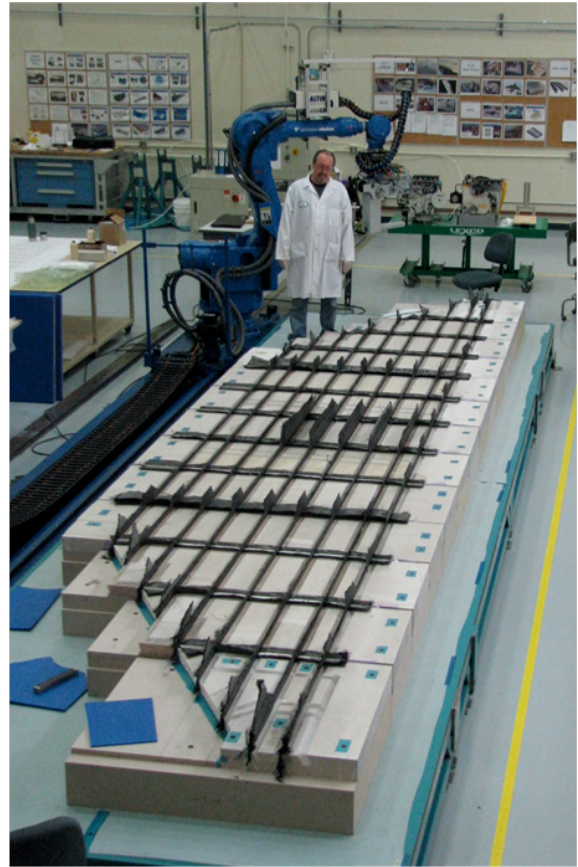
Figure 100. Preform Assembly Starts with the Inserting the Frames and then the Stringers
