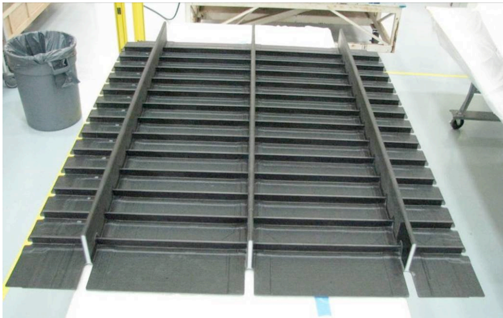
Figure 77. Finished Outer Rib Panel – IML Surfaces
