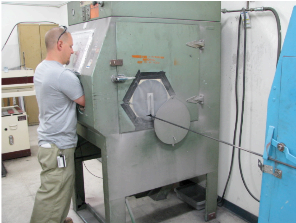
Figure 14. Grit Blasting of Rod to Prepare Outer Surface for Bonding
