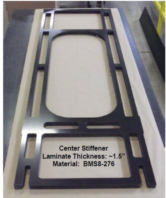
Figure 94. Trimming Solid Laminate Core Details
