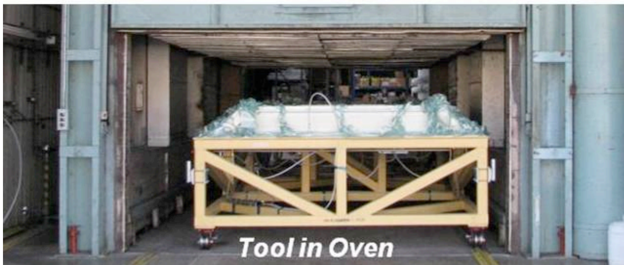
Figure 35. Part is Transferred and Loaded into Oven
