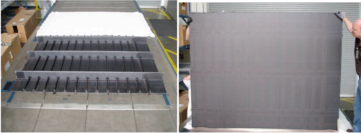
Figure 74. Second Untrimmed Cured Outer Rib Panel - IML and OML Surface
