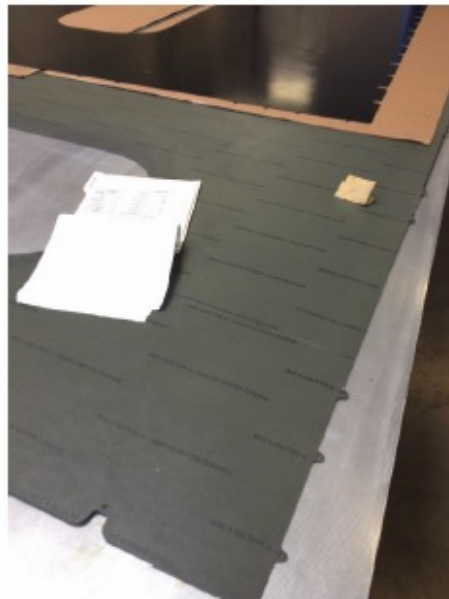
Facesheets fabricated with a peel ply on the surface that will be bonded
