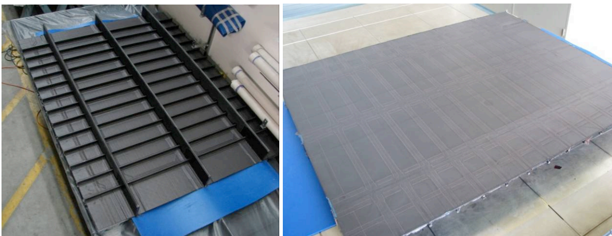
Figure 73. First Untrimmed Cured Outer Rib Panel - IML and OML Surfaces
