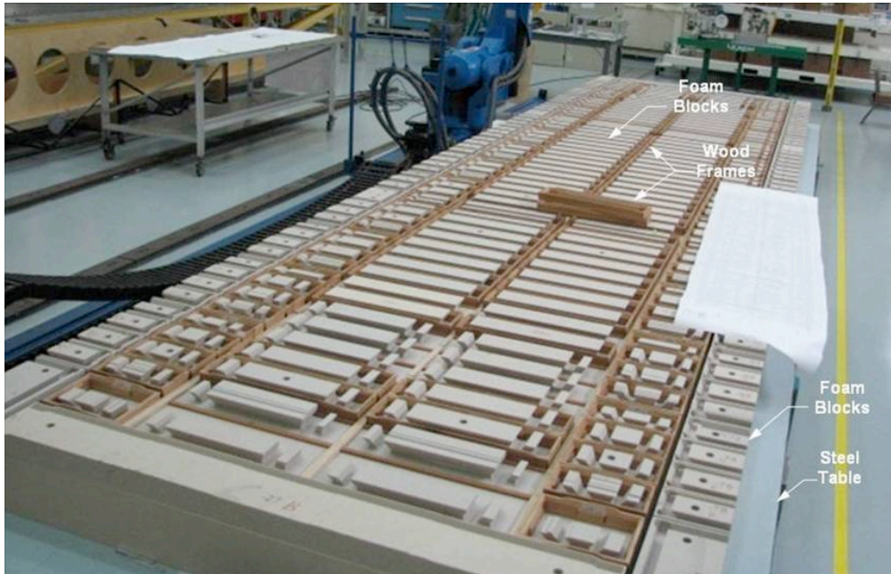
Figure 23. Crown Panel Stitch Tool Preparation and Checkout
