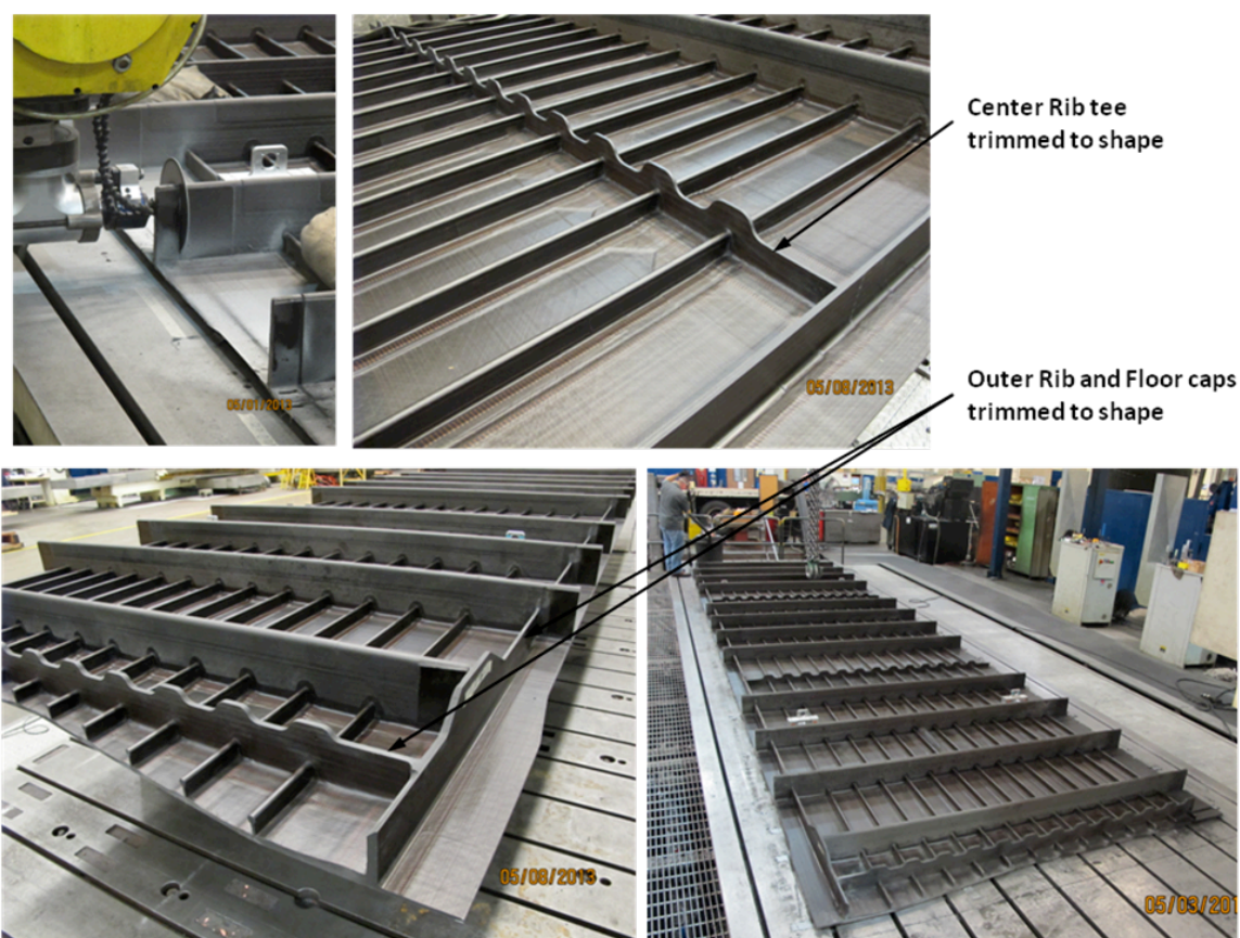
Figure 93. Upper Bulkhead Panel Trimming
