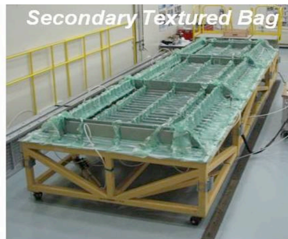
Figure 34. Secondary Bag is added to Maintain Vacuum Integrity during Infusion and Cure
