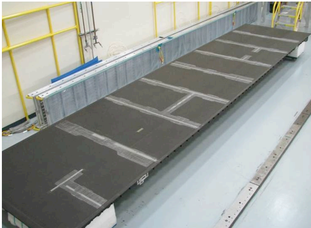
Figure 50. Bonding Surfaces were Readied for Repair Patches
