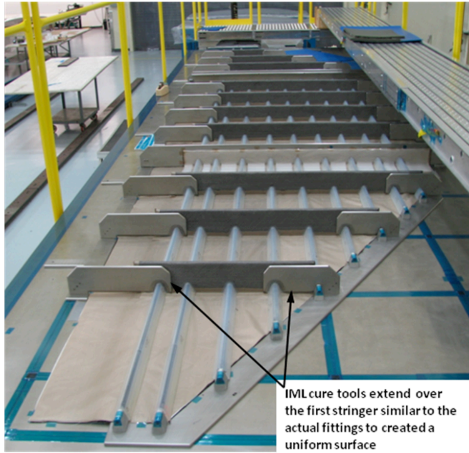
Figure 106. IML Cure Tool Positioned on the Preform
