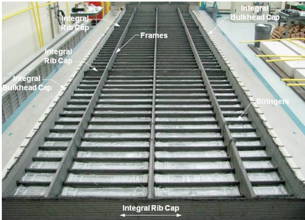
Figure 30. Self-Supporting Crown Panel Preform Placed on the Cure Tool
