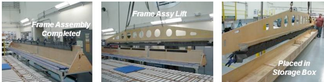
Figure 21. Completed Frame Lifted from the Frame Assembly Tool
