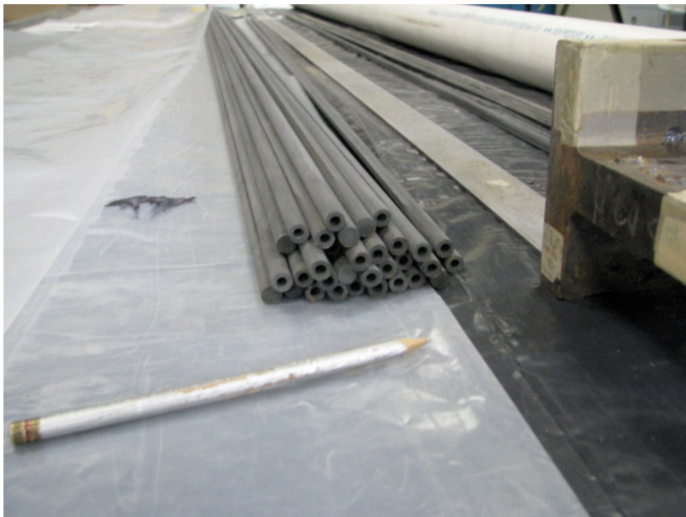
Figure 15. Prepared Rods Ready for Deionized Water Rinse and Water Break Test
