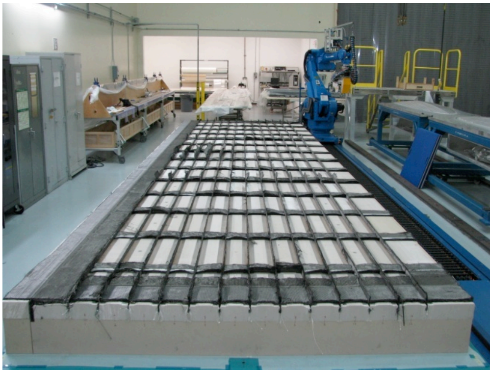
Figure 83. Upper Bulkhead Stringer Stacks Inserted into the Stitching Tool
