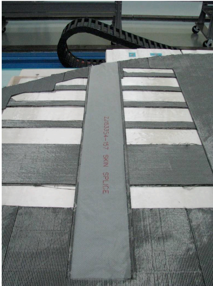
Figure 103. IML Skin Splice Straps are Located on the Preform Assembly
