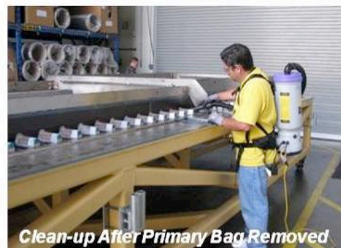
Figure 38. Bag and Tool Removal Prior to Post Cure
