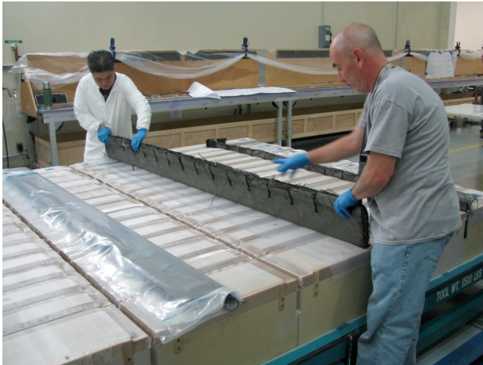
Figure 79. Frame Installation on First Upper Bulkhead Panel
