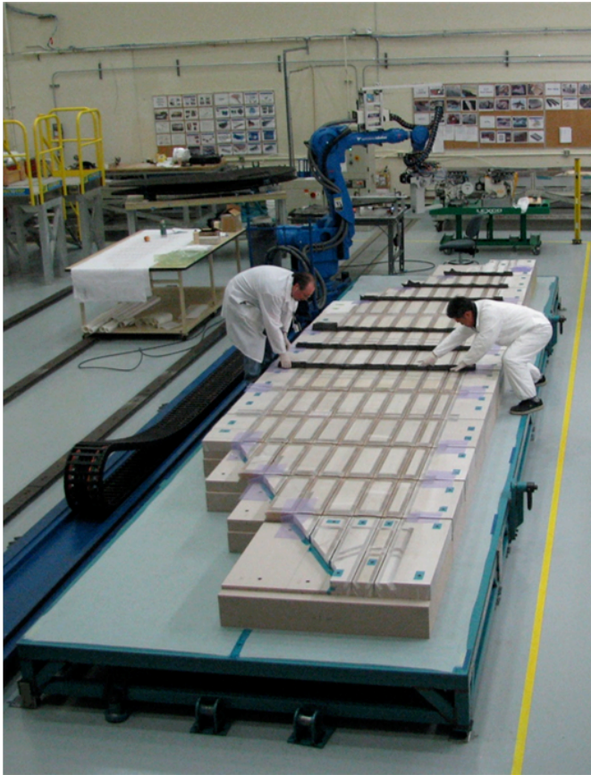
Figure 100. Preform Assembly Starts with the Inserting the Frames and then the Stringers
