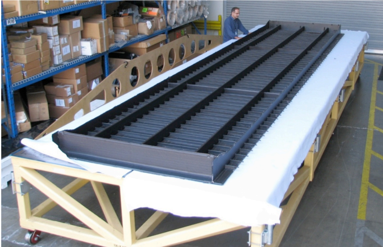
Figure 39. Final Cured Crown Panel Read for Edge Machining
