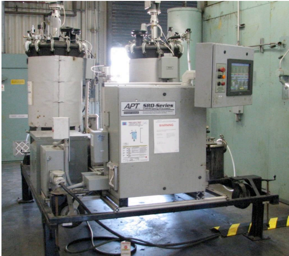
Figure 36. Automated Infusion Equipment Used for Resin Infusion
