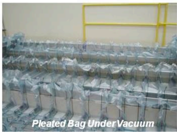
Figure 33. Pleating Operation for Primary Bag Installation
