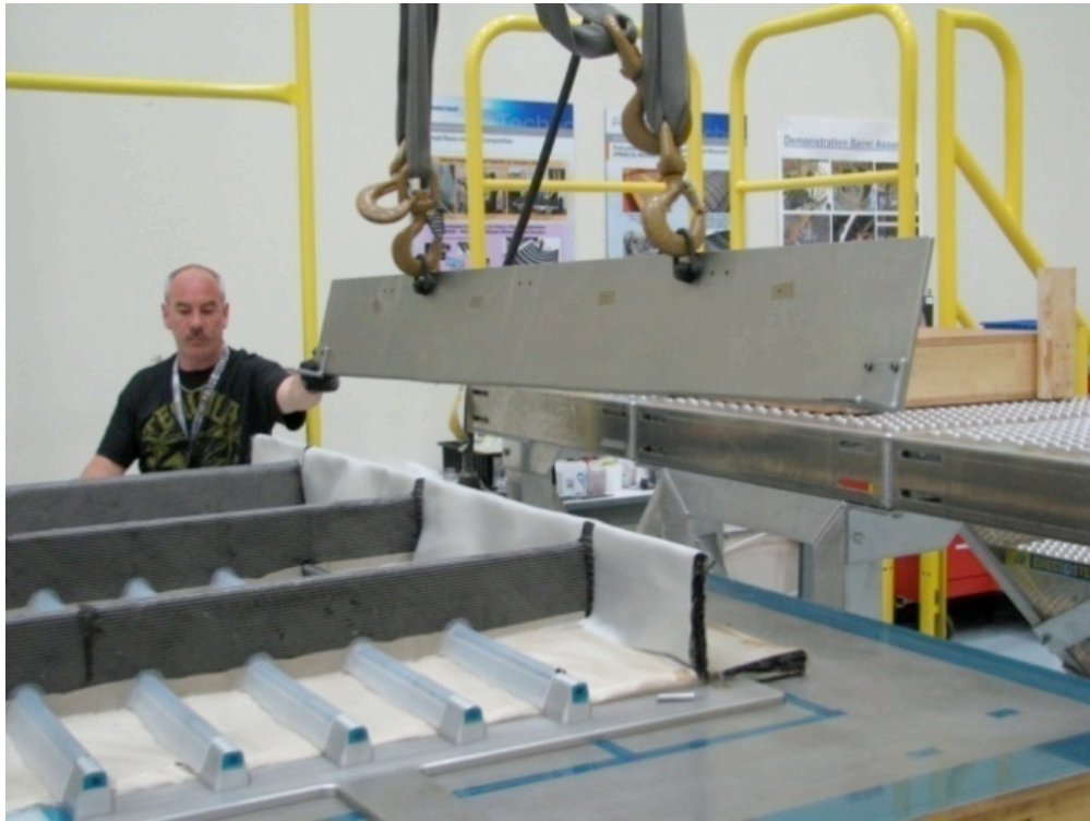
Figure 56. Integral Cap Tooling Plate Installation
