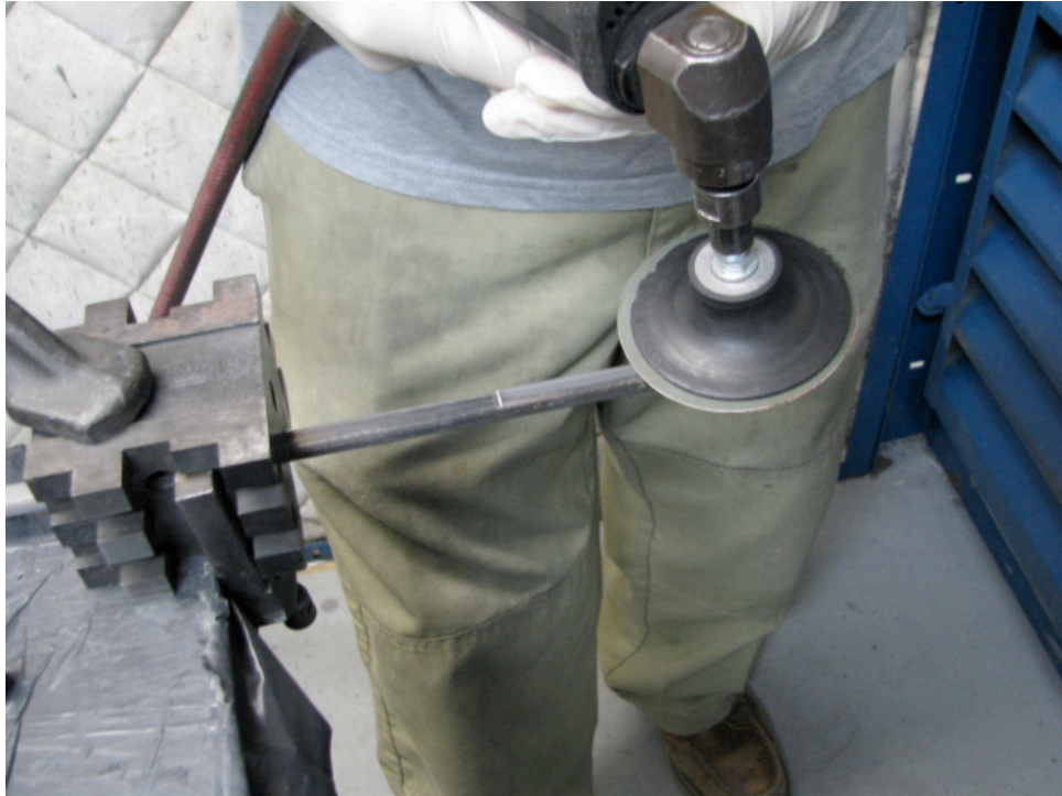
Figure 12. Removal of Fillet Feature from End of Rod Using Abrasive Sanding Disk
