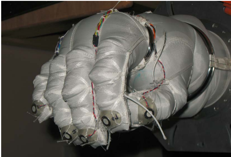
Figure 1. GECO Pressure Glove with Vibrotactile Actuators
