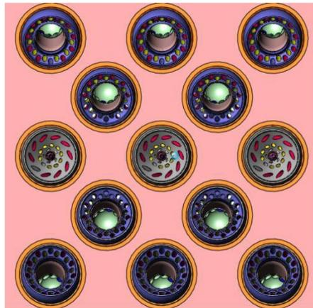
Figure 3.—Multi-Point Array with air blast fuel injectors.
