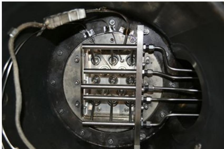
Figure 15.—MLDI combustor installed in the Medium Pressure Rig at UC.
