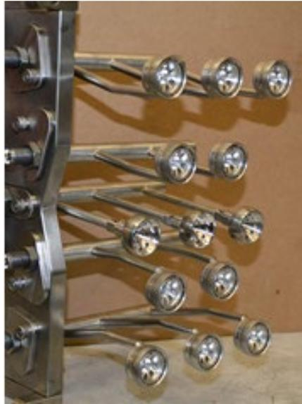
Figure 12.—Fuel injector assemblies for Medium Pressure Rig testing at UC.
