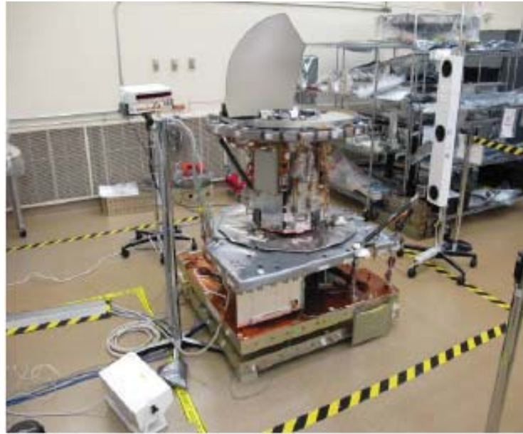
Figure 1. Dynamometer Assembly Setup in Calibration and GMI without RDA and MR Assys Integrated
