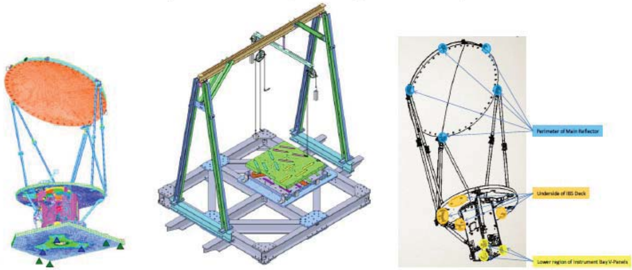
Figure 2. (a) Structural Model of the GMI Instrument Assembly, (b) Dynamometer with the Spin Balance Test Fixture, and (c) Balance mass locations on GMI
